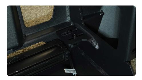
STEP 18 | If you are planning on running pod lights we, install the lights now using the hardware provided with the light.
