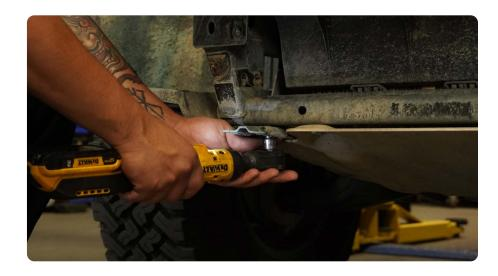
STEP 9 | Use a trim clip tool to remove the clips that secure the lower shutter air scoop to the vehicle.
