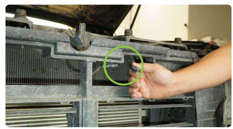
STEP 11 | Use a 10mm socket to remove the (8) factory bolts that secure the upper radiator shutter assembly to the vehicle.
