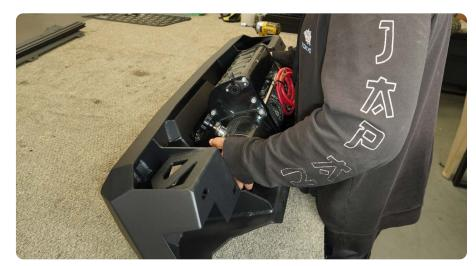
STEP 21 | Lift the bumper up to the vehicles frame rails. Using the factory crash-bar hardware, loosely secure the bumper to the frame rails.
