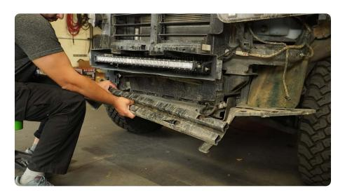
STEP 7 | Use a 18mm socket to remove the factory recovery hooks.
