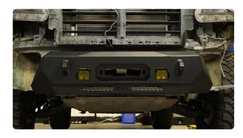
STEP 22 | Use the provided M8 Nut plates and the provided M8 hardware to secure the winch plate to the vehicles bottom radiator support bar.
