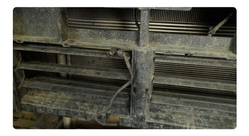
STEP 15 | With the bumper/grille on a covered work area face down, unclip the factory clips that secures the bumpers center section.
