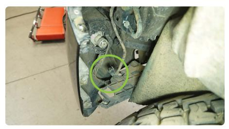
STEP 5 | Remove the bumper/grille assembly from the vehicle with a firm grip
