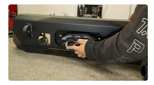
STEP 20 | If planning to run a winch, install the winch now.
