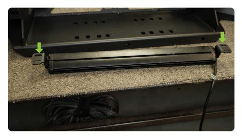
STEP 17 | Mount the light bar onto the bumper as shown. Use the provided M6 allen head hardware to secure the light bar to the.
