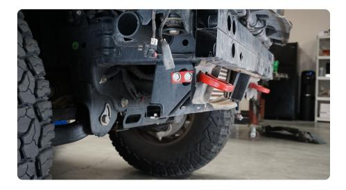
STEP 11 | Use a 7mm socket to remove the bolts that secures the shutter shroud to crash bar.
