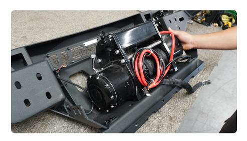
STEP 21 | Install the cover mounting plates using the provided tapered M6 hardware and an #4 Allen as shown.
