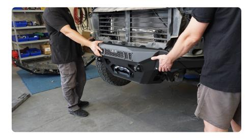
STEP 35 | Reinstall the recovery hook using the provided M12x80 hardware, ensuring the bolts thread through the winch plate support brackets as shown.
