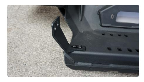
$\begin{array}{c|c} \text{STEP 16} & \text{Apply the provided peel} \\ \text{and stick foam pieces on to the bumper} \\ \text{wings as shown.} \end{array}$
