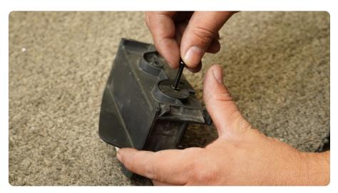
STEP 31 | With the bolt inserted, press on the backside to score the housing and using the 3/16": drill bit, carefully drill though to allow the bolt to be through bolted.
