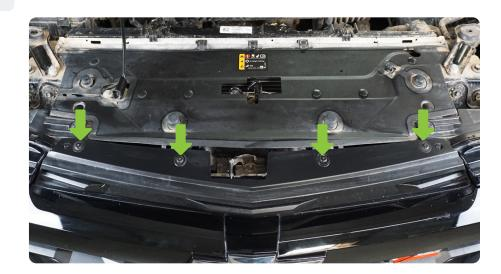
STEP 2 | Use a T15 torx tool to remove the torx head bolts securing the inner fenders to the front bumper.
