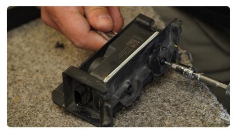
STEP 33 Once the assembly is complete, slide the motor into the mount on the skid plate and secure with two M6 bolts and nuts using a #4 and 10mm socket.
