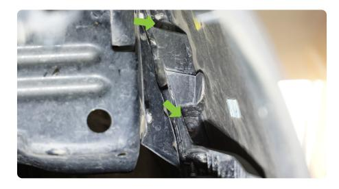
STEP 4 | With a firm grip, separate the bumper from the fender.
