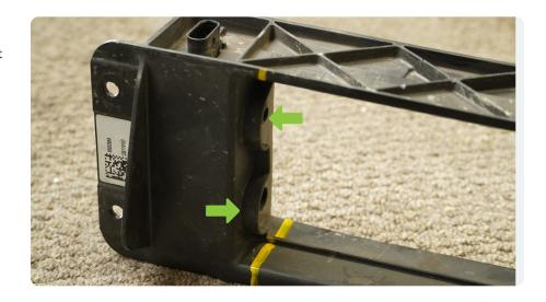
STEP 27 Once marked, cut the motor housing away from the structure using a grinder or similar cutting tool.
