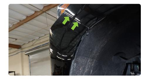
STEP 45 | Use a T15 torx tool to secure the inner fender to the bumper/grille assembly.
