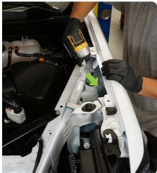
STEP 6 | Carefully start to pull the lower fascia away from the vehicle with a firm grip.
