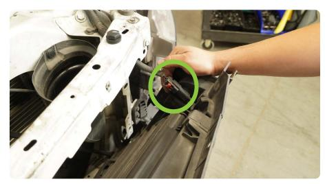
STEP 10 | Disconnect the bumpers wiring harness located below the passenger headlight. Pull back the red locking tab and depress the push tab to separate the two electrical plugs.
