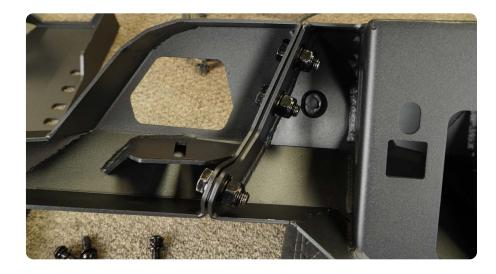
STEP 29 | If running a 20" dual row light behind the mesh, use the provided M6 hardware to loosely secure the provided brackets.
