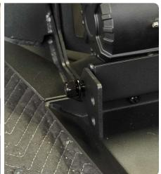
STEP 27 | Place the provided foam onto the mating surface of the bumper or wings as shown.
