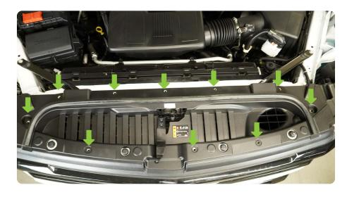
STEP 3 Using a 10mm socket, remove the (4) bolts securing the top of the grille to the vehicle.
