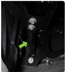
STEP 12 | Use an 18mm socket to remove the (2) lower bumper mounting bolts on the inside of the frame rails.
