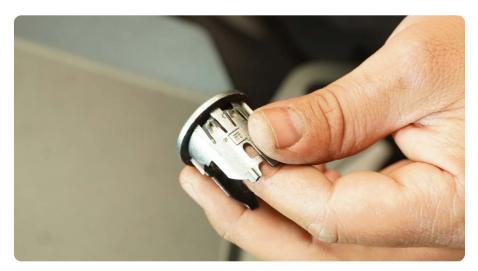
STEP 32 | Install the sensor bezels into the DV8 front bumper by pressing them into the bumper from the front side.
