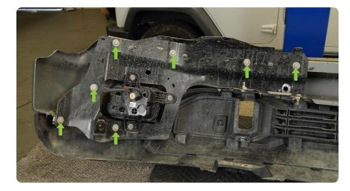
$\begin{array}{c|c} \text{STEP 21} & \text{Using a trim tool, remove} \\ \text{the clips holding the harness to the} \end{array}$ bumper.
