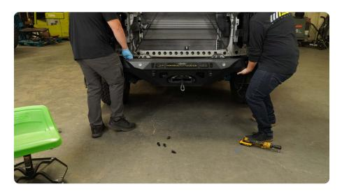
STEP 37 | Use a 18mm socket to secure the bumper in place and reconnect the bumper harness.
