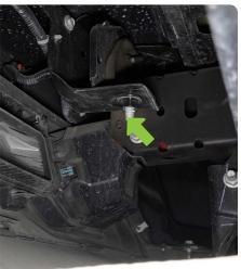
STEP 13 Use a 10mm socket to remove the (4) bolts securing the bumpers lower valance.
