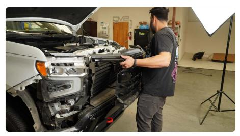
STEP 8 | If your vehicle is equipped with an illuminated grille emblem, disconnect the (2) electrical plugs behind the driver side headlight.
