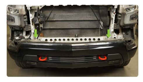
STEP 15 | Use a 15mm socket to remove the (6) bolts that secure the factory bumper mounting plate to the frame rails.
