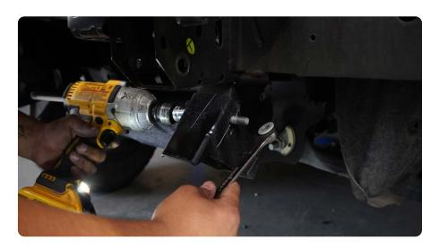
STEP 18 | Use a 10mm socket to remove both front inner fender supports.
