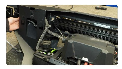
STEP 34 | Before installing the sensors, unwrap the harness tape to remove the wire stiffener.
