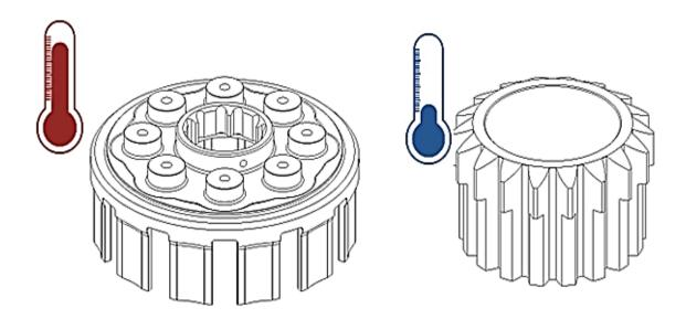
6. After 15 minutes, use oven mitts to remove the basket from the oven, then remove the starter gear from the freezer.
