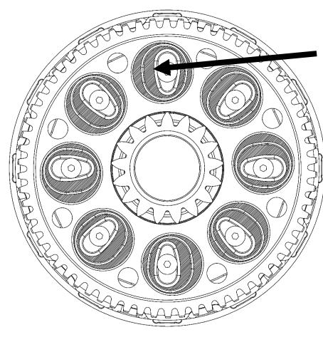
Starting from the top install dampers with the thick side of the damper to left of the standoff 11. Reinstall the OE ring gear (recessed side out). The ring gear may fit snugly and will likely require using a soft mallet to tap it on until it seats down against the basket.
