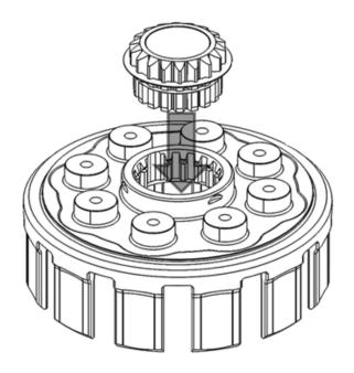
9. Once the gear is far enough into the basket that the ziptie starts to deform, pull the zip tie out before pressing the gear fully into the basket.
