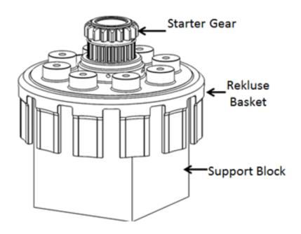
8. Quickly align the frozen starter gear, then slowly press it into the basket, making sure the snap ring is seated in its channel. **Be careful not to touch the hot basket.**
