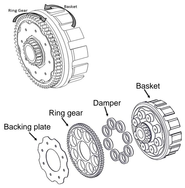
2. If any rotational play can be felt between the basket and the ring gear, the dampers are worn and either the dampers and/or basket assembly need to be replaced.
