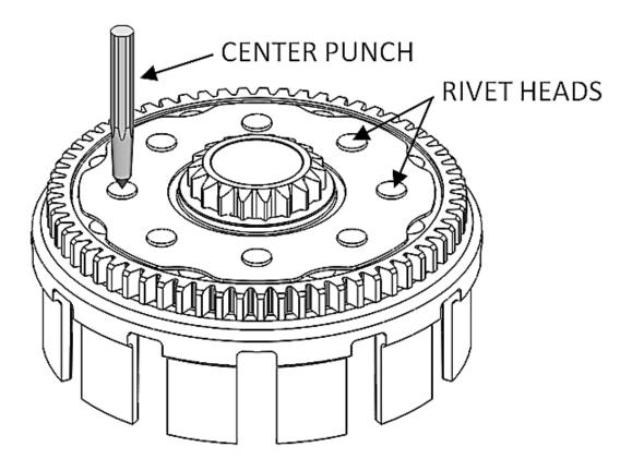
4. Using the supplied drill bit, drill out the heads of all the rivets. Set your drill to 300-400 RPM and use proper cutting fluid or oil for best results.
