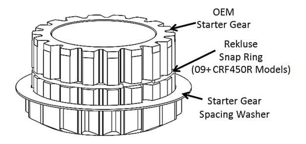
3. Secure a tip-tie over the snapring to hold it in place during installation.
