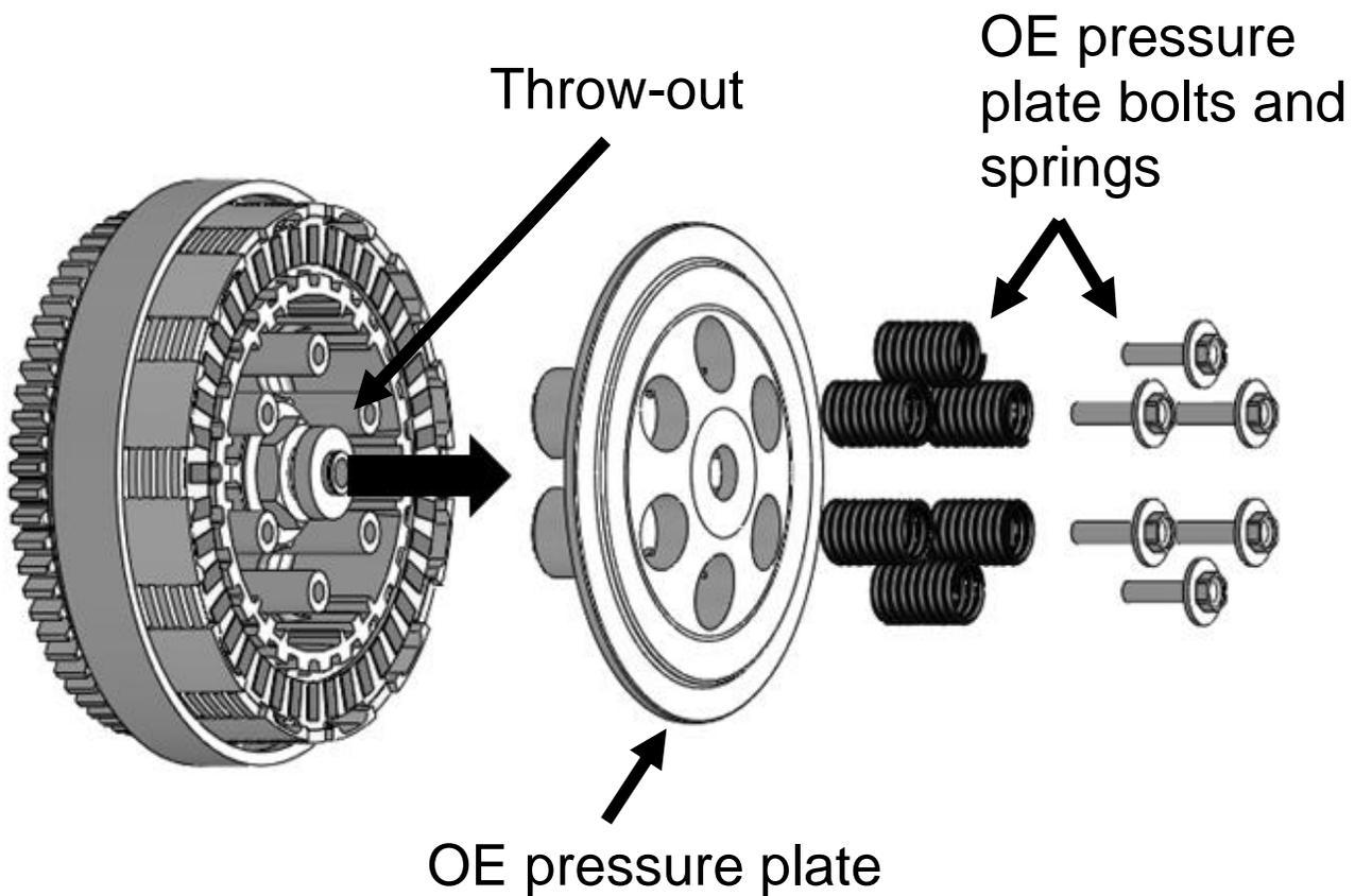
**Note:** *Throw-out washers can stick to the back of the pressure plate. Be sure to reinstall any throw-out washers back onto the throw-out.*
