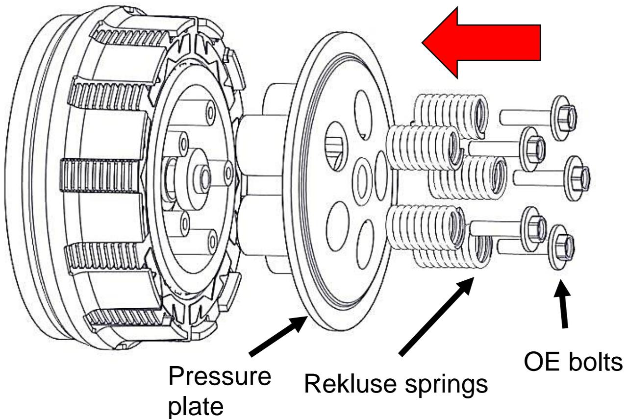
**Note:** *For Yamaha YZ250F (2019+), YZ250FX (2020+), & WR250F (2020+) when installing the pressure plate align the indent in the pressure plate with the indent in the center hub.*
