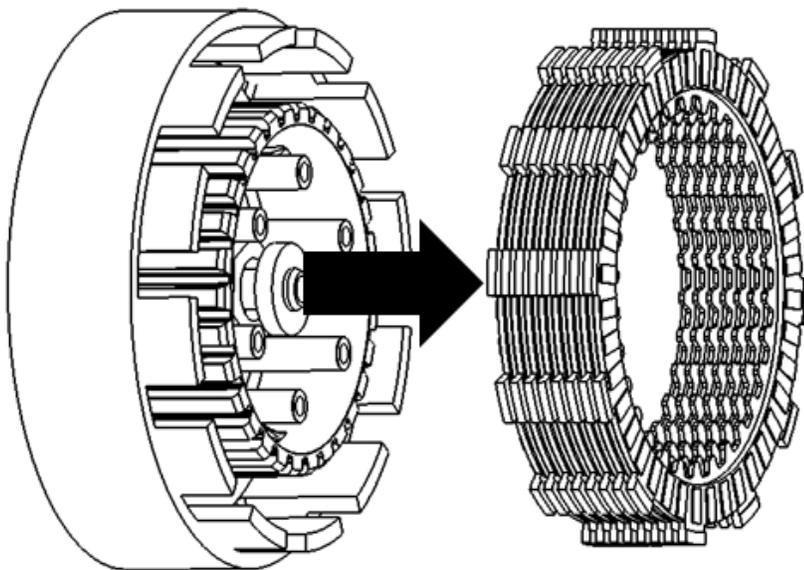
**Note:** Some models have a clutch judder (boss) spring located in the bottom of the OE friction pack. This consists of a spring, seat and narrow friction. If your bike is equipped with these parts, remove them and set them aside.
