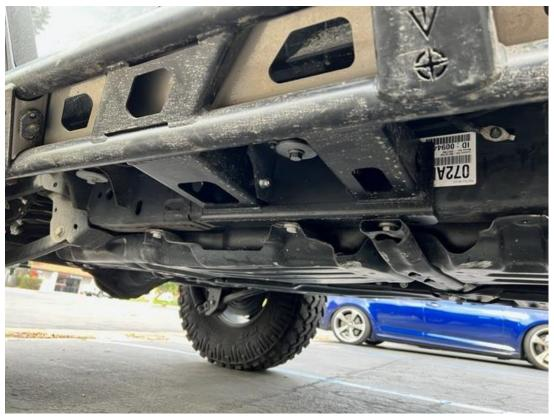
Press slider up towards frame to fully seat against it. Install the removed factory bolts back into their original bolting locations. Snug bolts (Will be removed again later).
