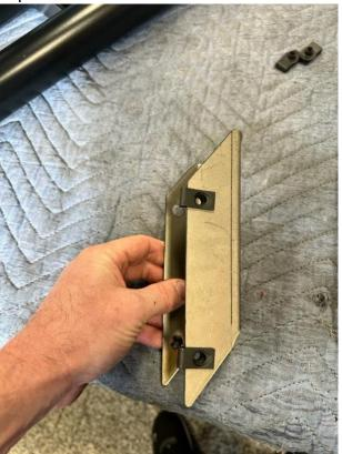
Lighting. Insert light wire through hole in end cap. Install light to bracket using supplied M4 bolts.
