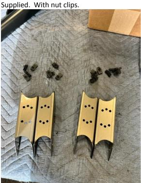
End Plate Assembly: With a firm push, press on nut clips to Slider End Caps over the 4 holes of each part. Barrell section of nut clip should be on the inside of the part all 4 places. Center clip thread over holes.
