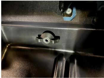
**STEP 6:** Re-install the jack on the studs, use your 10mm deep socket and tighten the nuts till they are snug. Do not over-tighten, it could possibly rip the plastic tray. On the opposite side, re-install the plastic nut removed from the lug wrench bracket in previous steps, do not over-tighten.
