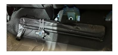
**STEP 3:** Remove the factory lug wrench and set aside. After the tray is installed, this will be the first item stored in your new underseat storage.
