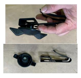
**STEP 4:** Separate the plastic nut from the lug wrench bracket. Press down on the tab pointed to in the top picture and slide plastic screw out.
