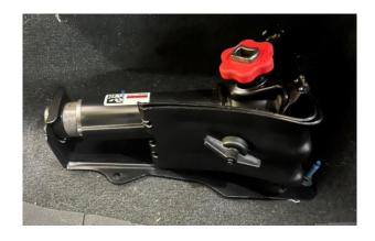
**STEP 2:** Using a 10mm deep socket wrench, remove the two nuts holding down the factory jack and move the jack out of the way for tray installation. You will re-install the jack and nuts at a later time.
