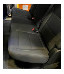
**STEP 1:** Lift up factory rear seat and clear out any loose items/debris. The factory divider will remain folded down for storage tray installation.
