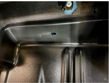
**STEP 5:** With the jack and lug wrench removed, it is now time to install the storage tray. The factory studs should match up with the pre-made holes.
