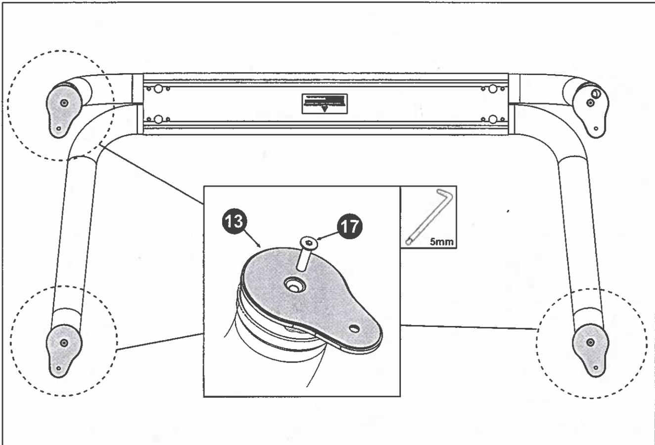
7. Install the remaining Mount Brackets (13) to the Sportsbar foot ends over the Foot Cups and secure using the M8 Countersunk screws (17).
