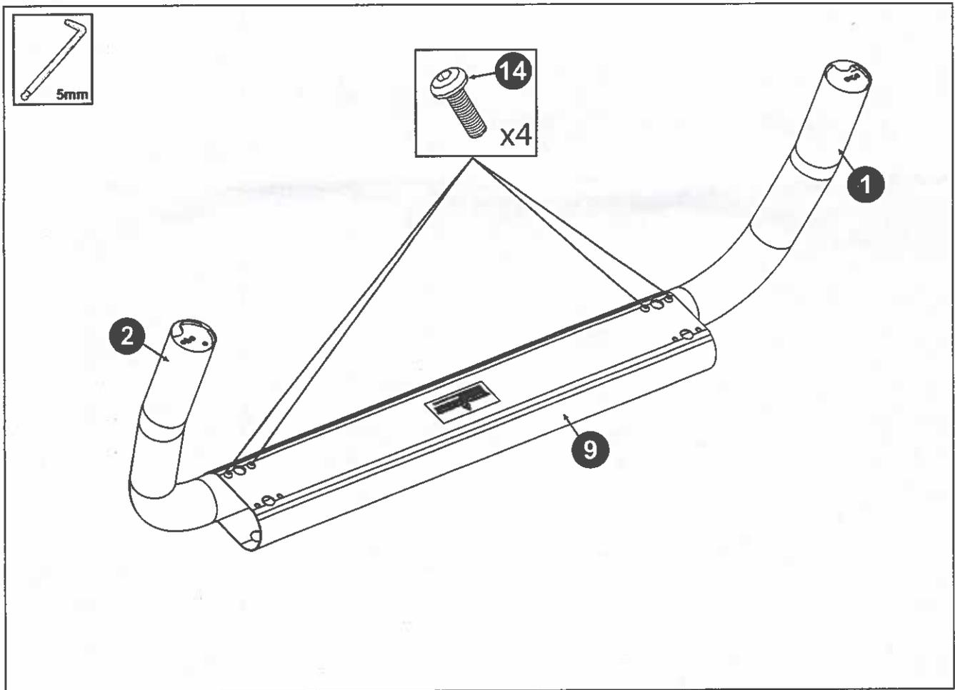
2. Position the Center Piece (9) on a soft surface or mat with the warning label facing towards you as shown. Install the LH Front Leg (1) and the RH Front leg (2) into the forward half of the Center Piece (9) and loosely fasten M8 Hex Pan Head Screws (14).
