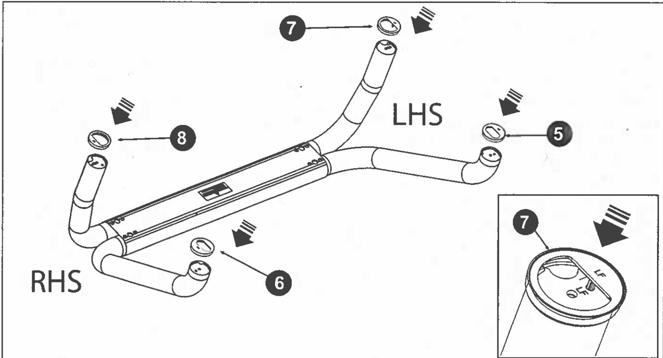
5. Push all four rubber Foot Cups onto the corresponding foot of the Sportsbar by aligning the Foot Cup leg to the tube as shown.
