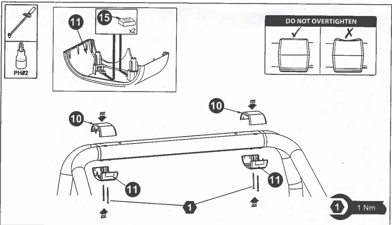
16. Insert M5 Square Nuts (15) into the Upper Cover Cap (10). Install the Cover Caps - Upper (10) and Lower (11) halves to the Centre Piece (9) and fasten together using M5 x 85mm Pan Head Screws (16). Torque the Screws to 1Nm. NOTE: Do not overtighten.
