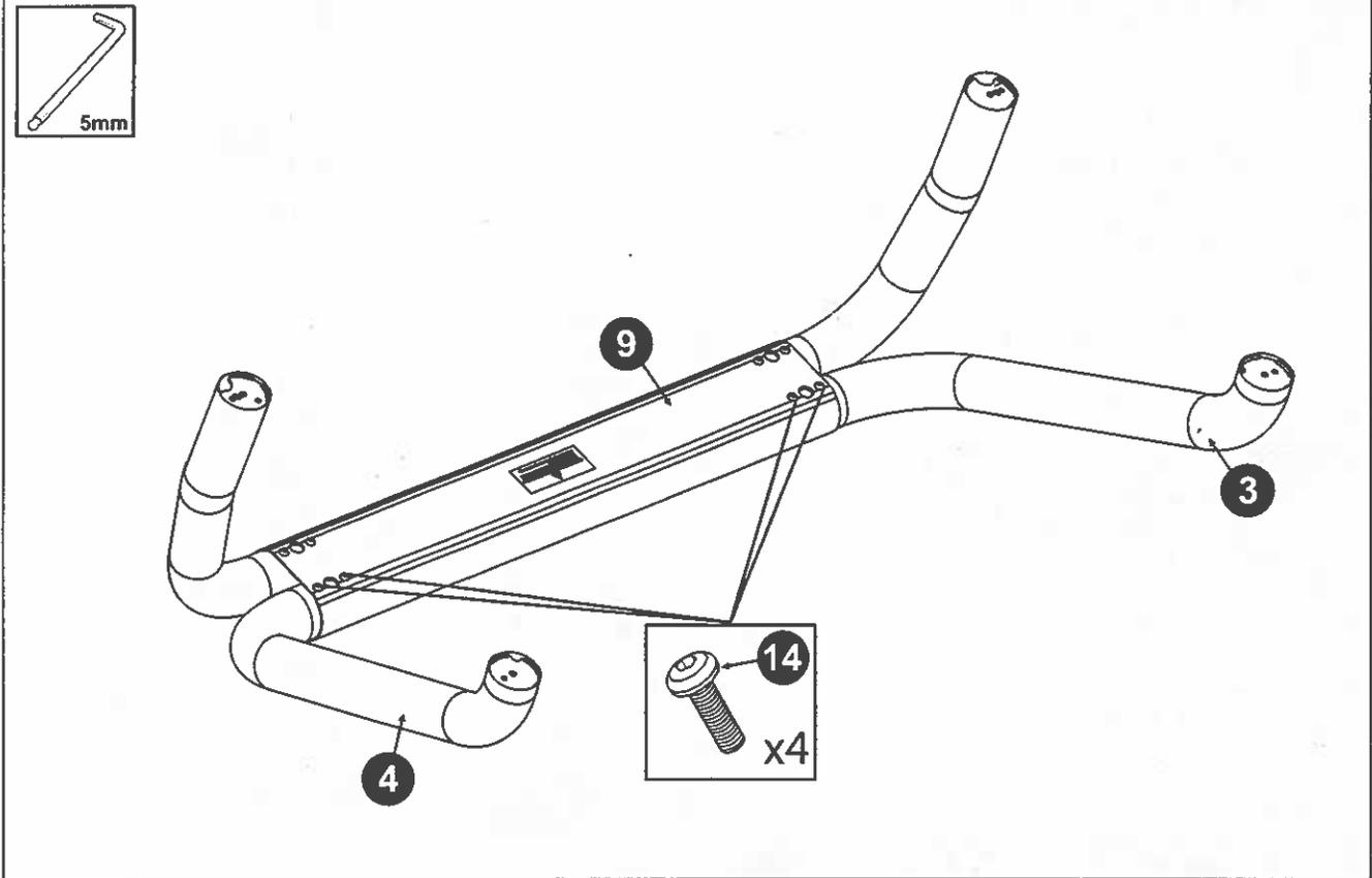
3. Install LH Rear Leg (3) and RH Rear Leg (4) into the rear half of the Centre Piece (9) and fasten using M8 Hex Pan Head Screws (14).
