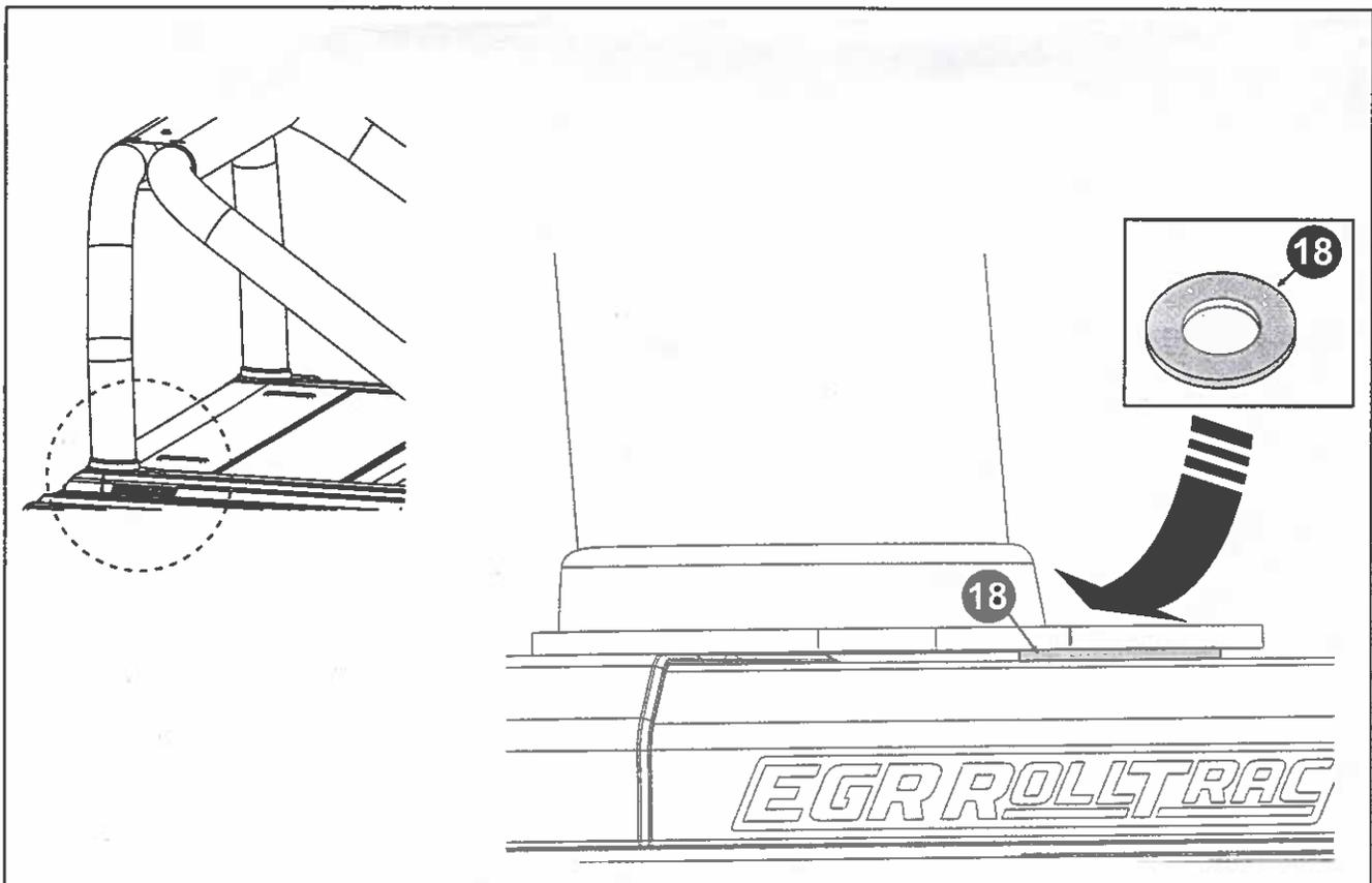
12. Slightly lift both front end legs of the Sportsbar and place the Large Washer (18) under the Front Mounting Brackets as shown. Ensure the Large Washer (18) hole aligns with the Front Mount Bracket holes and the side rail T-Channel.
