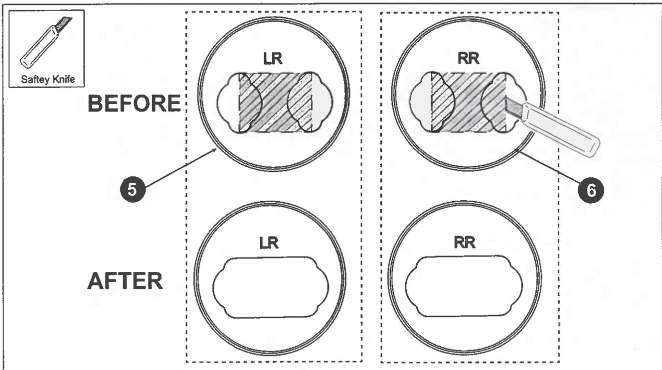
4. Locate the LH Rear Footcup (5) and RH Rear Foot Cup (6). Mark then cut the Foot Cups as shown and discard the cut out sections (shown above).
