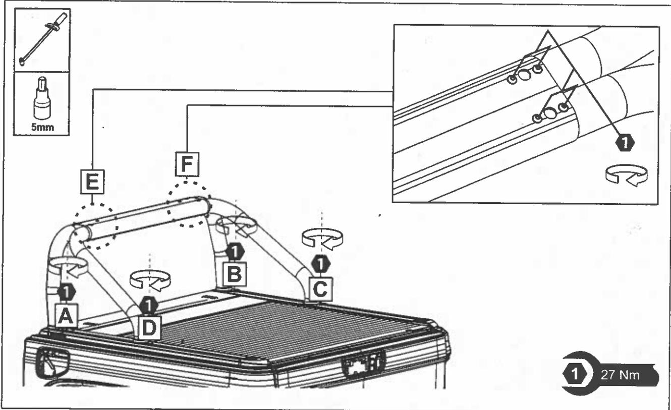
15. Tighten all M8 x 16mm Countersunk Screws (19) and M8 x 30mm Pan Head Screws (14). Follow carefully the order of torquing (A, B, C, D, E, F). Torque to 27Nm.
