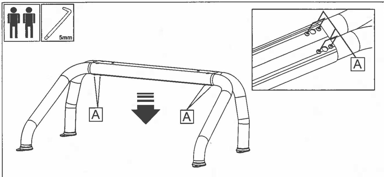
8. Using two people, carefully lift the Sportsbar and place it on a flat surface to make sure the legs are level. Adjust tubes if required by loosening the screws (A).
