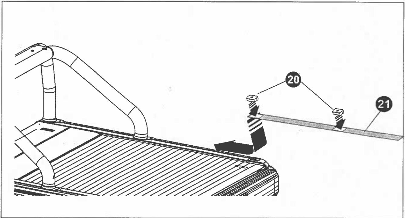
13. Insert the Installation Aid (21) into the T-Channel of the RollTrac side rail. Slide two Slot Nuts (20) into the T-Channel and position them on top of the Installation Aid.
