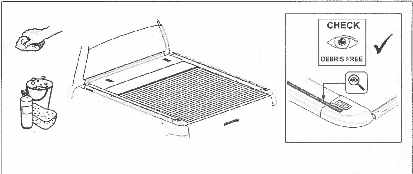
1. Prepare the surface of the RollTrac side rails by cleaning them thoroughly ensuring that any debris in the RollTrac side rail T-channels is completely removed.
