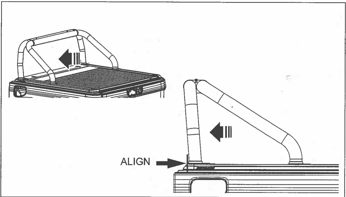
11. Position the Sports Bar such that the Front Mount Bracket Plates align to the RollTrac side rail End Caps as shown.
