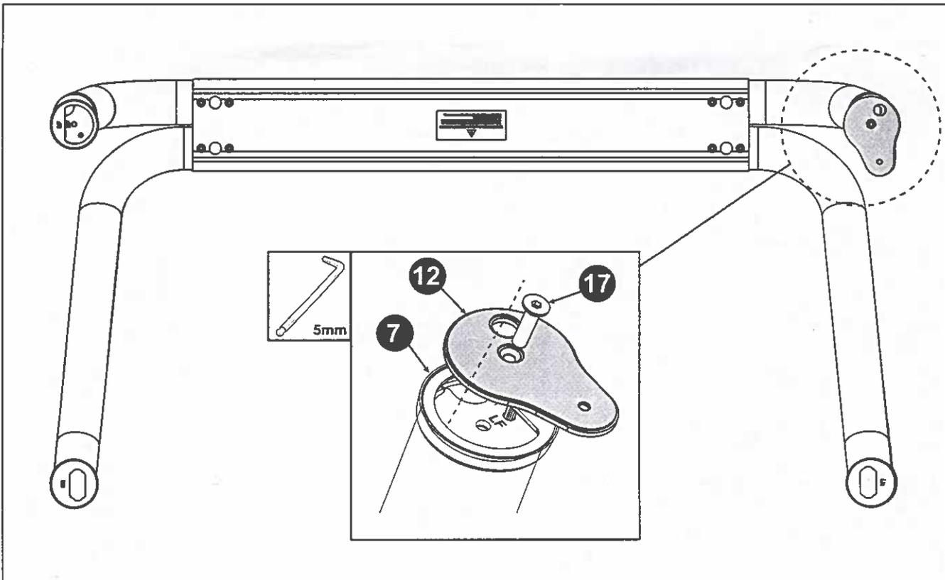
6. Install the Front LH Mount Bracket (12) (With Hole) by aligning the hole to the Sportsbar foot end over the Foot Cup as shown and secure using the M8 Countersunk screw (17).
