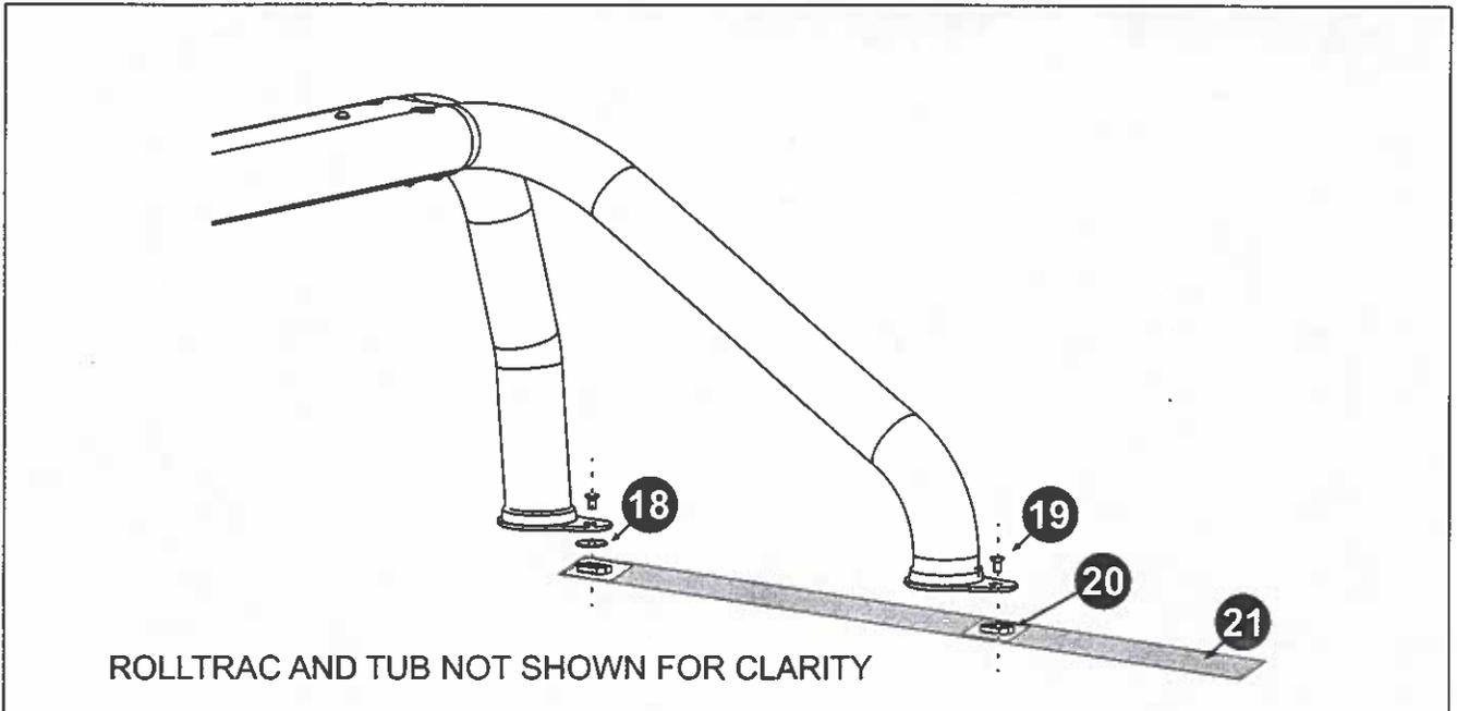
14. Reposition the Slot Nuts (20) inside the RollTrac side rail T-Channel using the Installation Aid (21) and align with the holes in the RHS Mount Brackets. Loosely install the M8 x 16mm Countersunk Screws (19) through the RHS Mount Brackets. Once both Screws are finger tightened, remove the Installation Aid (21) from the T-Channel and repeat for the LHS. Ensure the front Countersunk screw (19) passes through the Large Washer (18) as shown.
