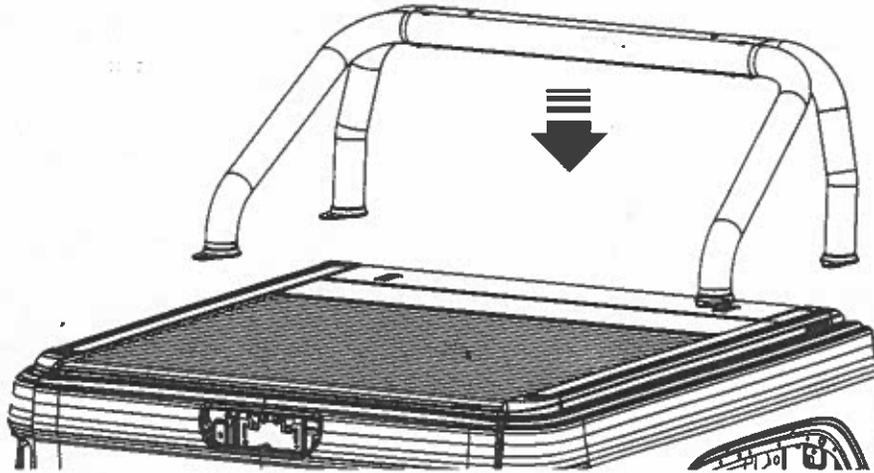
9. Using two people, carefully lift the Sportsbar assembly above the RollTrac and carefully lower the Sportsbar assembly over the RollTrac side rail.
