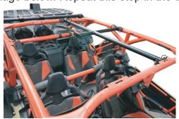
Once the structure is overlaid, 2 screws must be placed in the center of the structure to hold both parts. Tight all the nuts to the OEM specifications.
