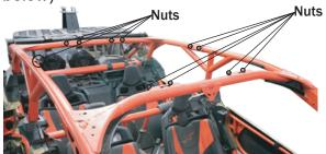
The passenger's side structure must be placed first, the central part of the "H" must fit in the screws that are shown in the image below. Repeat this step in the driver's side.
