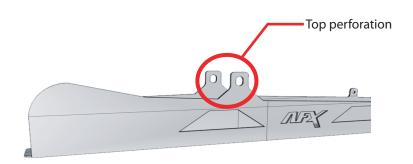
Insert the original screw into the top hole and one 1/4" x 2 1/2" screws in the perforations of the rear suspension thightening with double washers and one nut of 1/4".
