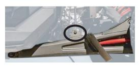
Place the rear suspension on the axle of the vehicle where the top perforation of the part matches the perforation of the screw that was removed (as show in the pictures).
