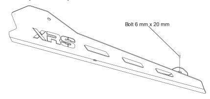
5 Adjust the slider on the side with washers and nuts provided (2 holes for 2 bolts on side).
