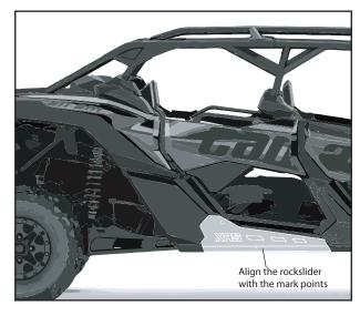
Remove the rivet/bolt underneath and use the 6mm x 20mm bolt to adjust the slider underneath the machine on the empty hole. (Place the slider between chassis tube and the plastic skidplate.
