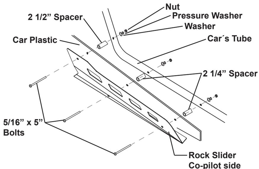
**4** Tighten the bolts to finalize the installation.
