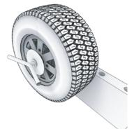
(Right side) Place one of the screw eye bolt on the washer and put it on the perforation of the spare tire carrier. (As shown on the image). Do the same step for the left side.
