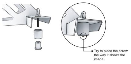
Align the Spare Tire Carrier with the perforations on the bed of your Ranger. Let space on both sides to put your tire.
