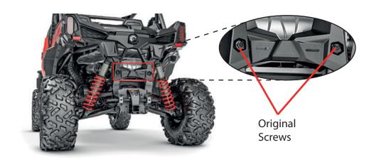
Use a two 5/16 x 1" screw with washer and nut and place it wheeit is indicated in the image. (do not thigten yet).
