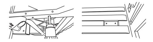
Use two (5/16" x 3") bolts on each side to secure the bumper brackets to the vehicle.
