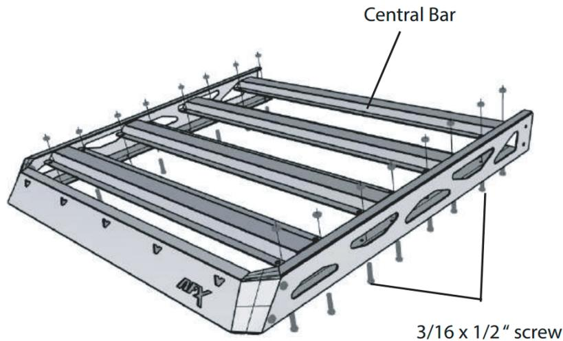
**5** Place the rear rack with the front rack, aligning the "C" hardware with the perforations (as it is shown in the image), using eight 1/4 x 1/2" screws with nut. (Do not tighten yet).
