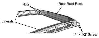
Place the front roof rack with the laterals (as it is shown in the image). Use four 1/4 x 1/2" screws with nut (Do not tighten yet)
