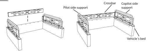
Join the crossbar with the 5/16" x 3/4" on both sides of the side racks and tighten all the screws.
