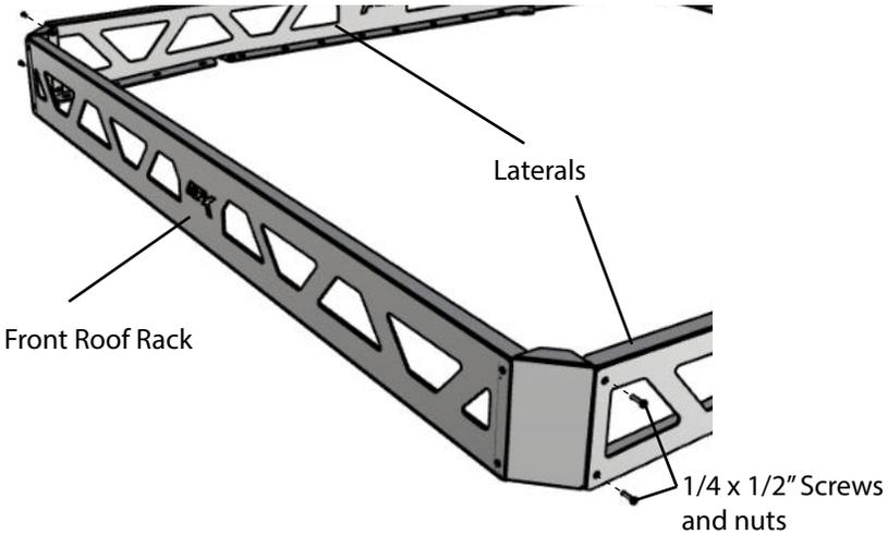
**3** Place the 8 central rails upward the front roof rack (as it is shown in the image).
