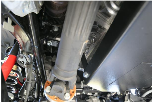
9. Install oil pan skid plate right/passenger side drop bracket in rear hole under motor mount hole using 1x 1/2" x 1/4" hex bolt with 1/2" washer and 1/2" nylock nut.
