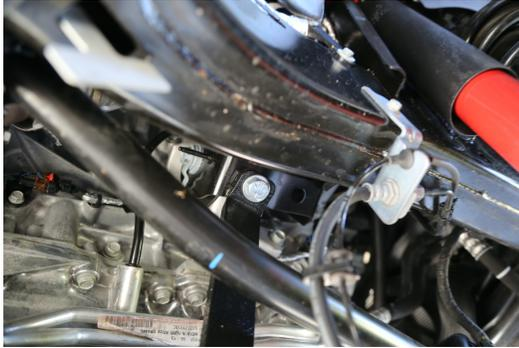
10. Mount rear of oil pan skid plate over belly pan skid plate (closest to ground) using 2x black bolts through oil pan skid, through belly pan skid, through cross member.
