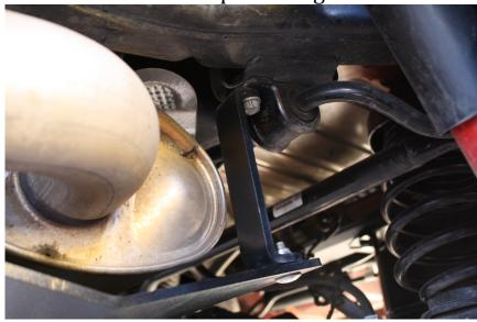
2. Install skid plate behind rear bumper and align mounting holes with existing frame rail holes. Using supplied bolt and washer, insert bolt through frame rail hole into skid plate mounting bracket. Use nut with welded tab. Leave hardware
