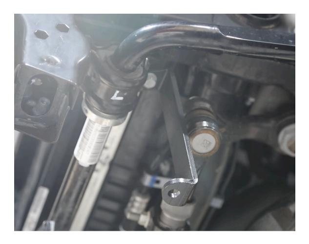
3. If factory nut is not installed inside lower frame supports in front of sway bar, use included welded nut tabs inserted into lower frame supports, held in place with piece of tape. The tape will hold the nut tab in place while inserting hex bolt.
