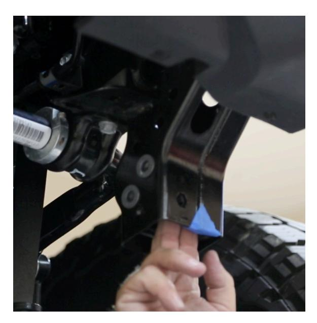
4. Insert hex bolt into front holes with washers to help hold skid in place. Install lower carriage bolts into skid, through bracket lower holes, with nylock nut on top. Once all 4 bolts are started, you can tighten all hardware.
