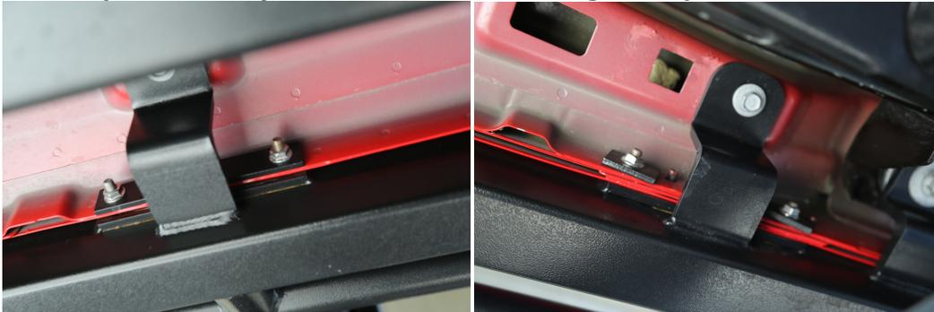
4. Reinstall factory body mount bolts with factory washers using 18MM socket OR use supplied replacement body mount bolts using 19MM with large black washers, do not tighten. If Gladiator, use longest bolts in 2 rear body mounts at truck bed.
