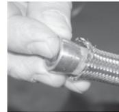
Push the brass ferrule around the Teflon and in between the braided hose. Seat the Teflon hose squarely against the bottom of the ferrule; this can be done by pushing the hose and sleeve against a workbench or vise.
