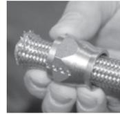
Install the threaded socket end on the hose and slide it back out of the way.
