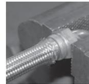
Follow by placing the hose end in a vise, sparingly lubricate the threads with 30wt oil or similar lubricant. Insert the hose over the nipple making sure the ferrule does not pop off the Teflon tube.
