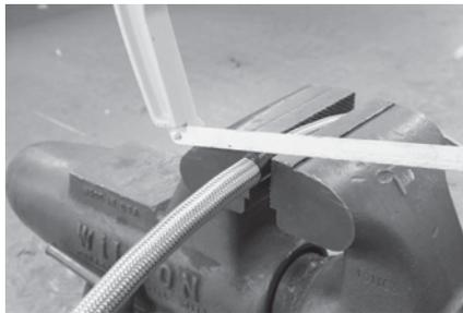
Start by tightly wrapping electrical tape around the hose in the area to be cut.
