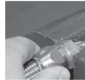
Finish by threading the socket end onto the nipple by hand.
