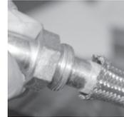
Insert the nipple portion of the hose end into the Teflon part of the hose to size it back up to shape then remove it.
