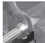
Now tighten with a wrench until the gap between the nipple and the socket is no more than 1/16".
