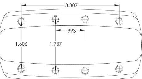
5. Install 1/4"-20 socket set screw in appropriate holes in billet pedal cover, install billet pedal cover on pedal then attach washer and lock nut. Tighten firmly by alternating turns at each nut with 7/16" wrench.
