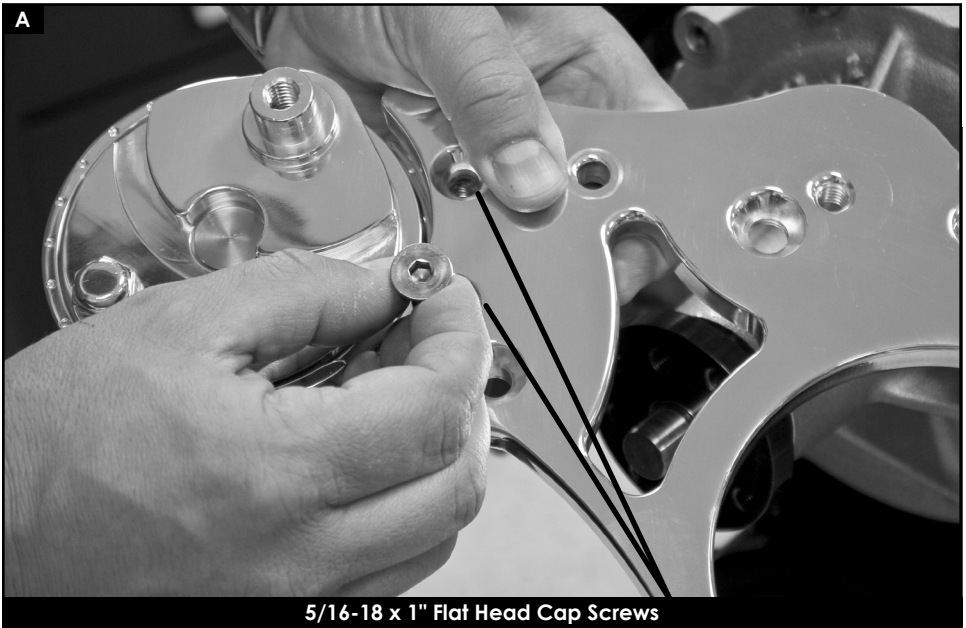
Figure 6: Install Tensioner To Bridge Bracket
