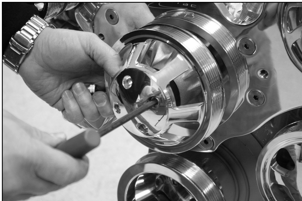
Figure 12: Install Water Pump Pulley
