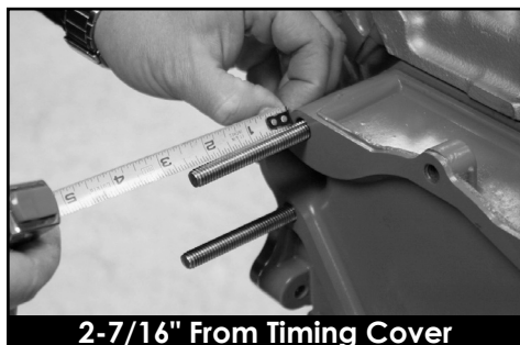
Figure 2: Install Block Mounting Studs
