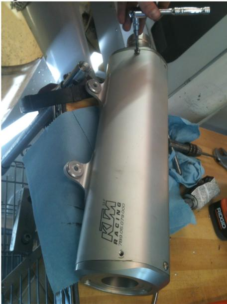
7. Install the new spark arrestor base; make sure that the base is pushed up tight to the muffler. Install one self-tapping screw at a time by drilling a 13/64" hole at each rivet location. Each time you drill a hole and install a self-tapping screw make sure that the base is pushed up tight to the muffler. **We recommend using lubricant for the self-tapping screws.**
