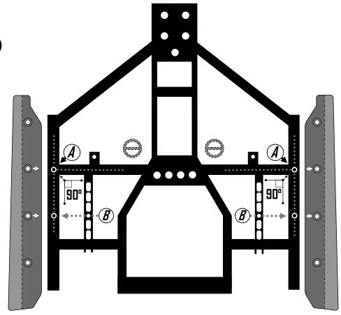
Ensure each mounting hole is drilled in to the center of the "Round" chassis tubing.
