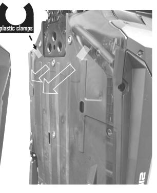
Install Rock slider Mounting Bracket through mounting holes in chassis frame, Ensure L and R are on the correct side, with larger end forward.
