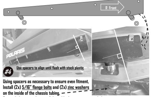
Fasten bolts securely, use of thread locker is recommended.
