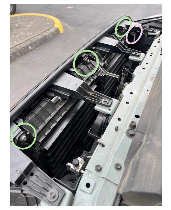
Reinstall the shutter assembly, using the factory three mounting locations at the top of the grille. Ensure connector is reconnected.
