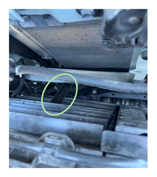
Ensure clearance of the grille supports through the shutter assembly
