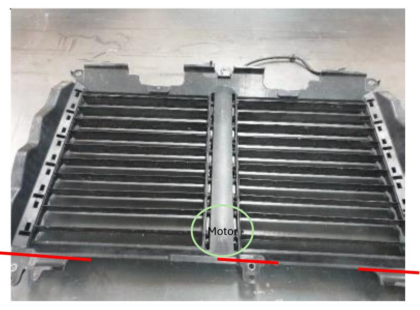
IF required, trim off the lower mounts for additional clearance, shown in RED
