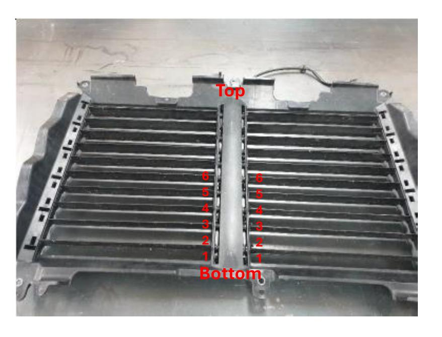
Counting up from the bottom, remove fins 4 & 5 from both sides
