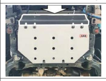
If fitting an ARB Bull bar, the stone panel is not required, skip to step 8.
