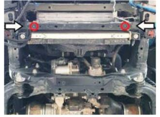
4. Insert a nut plate into each side of the front crossmember and align with the outer most holes on the crossmember.
