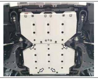
Install the Differential Panel using the four supplied M8 Flange bolts into the four threads in the chassis from the OEM panel locations. Torque to specification.
