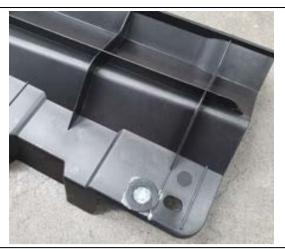
9. Using one of the supplied M8 Washers as a template, mark around the centre of the hole, repeat on other side.
