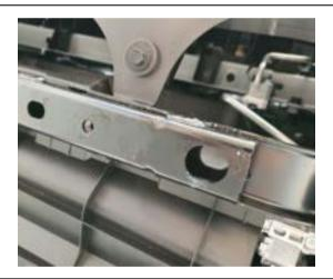
11. Re-attach the lower plastic air dam to the top of the crossmember with the OEM plastic scrivets.
