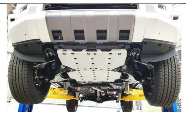
The Toyota LandCruiser Prado 250 Under Vehicle Protection Front Kit (5421240) is now installed.
