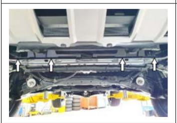
8. Remove the plastic scrivets with a small flat head screwdriver to remove the lower plastic wind dam.
