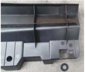
Using a utility knife or multitool, cut out the marked area as shown, repeat on the other side.
