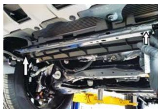
7. Using a white paint marker, mark the hole centres on the lower plastic air dam through the outer most holes in the front cross member as shown.
