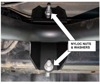
12. Use M12 washers and nyloc nuts to secure the mounting as shown
