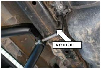
11. Insert U bolt between chassis and fuel tank, assemble it through the rear step mount. (6151785).
