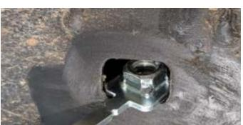
8. On the chassis in line with the middle rail mount, remove the plastic plug to expose the hole.
