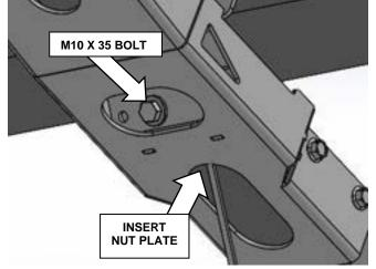
15. Attach the front mount to the chassis at the side using an M10 x 35 bolt, M10 flat washer and M10 nut plate. (3194639R)
