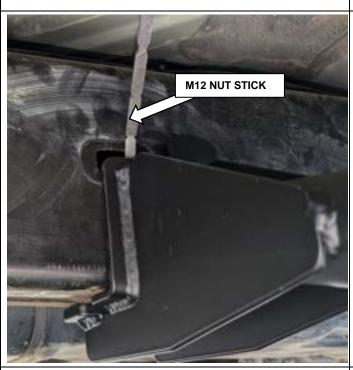
Assemble M12 x 30 bolt and washer into the M12 nut plate to attach the middle mount to the chassis
