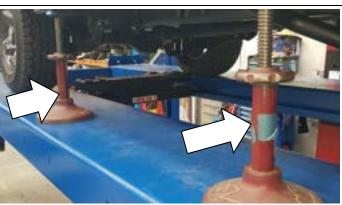
7. Place the RH Side Step against the chassis, Use adjustable axle stands or a second person to hold the rails in place.
