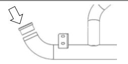
2. Fit the Rubber Plugs into the ends of the Side Steps.
