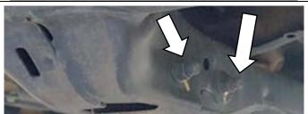
Support the gearbox crossmember. Remove Two OEM M10 nuts and bolts. Retain the fine thread OEM nuts for reuse.
