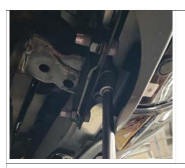
11. Carefully peel back bumper to access five fasteners retaining bumper bracket to crash beam. Remove and retain fasteners.
