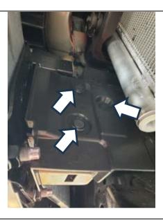
4. Remove two scrivets and one clip retaining air deflector moulding. Retain for refitment.
