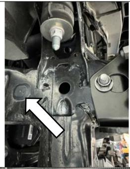
8. Remove outer plastic cap on third chassis hole. Retain for refitment.
