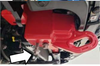
19. Loosely install M12 fasteners removed in Step 1.
