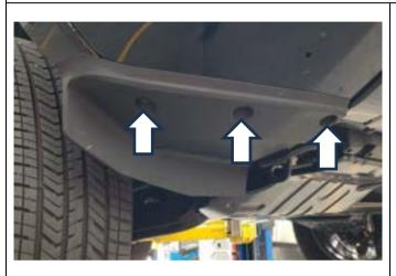
2. Remove OEM splash panel by undoing three screws from underneath and unclipping three scrivets from the wheel arch liner. Retain for refitment.
