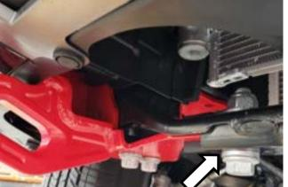
21. Identify bush and assemble bush up through the crossmember and the plate as shown.
