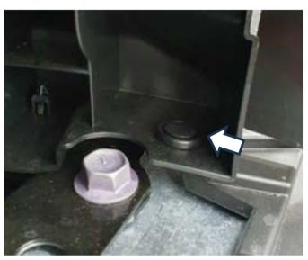
Using a short flat blade screwdriver remove the scrivet on top of the crash beam.
