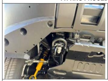
Remove tow hooks on the side the recovery point is to be fitted. Retain fasteners for refitment.
