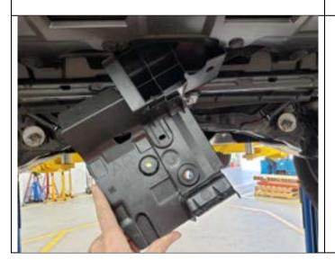
6. Carefully manoeuvre the air deflector to the middle of the vehicle and then lower to remove. Retain for refitment.
