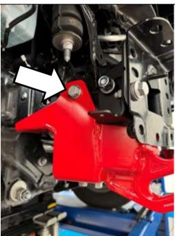
18. Loosely assemble M12x1.75x110 bolt, nyloc nut and hardened washers through the crush tube installed in step 15.
