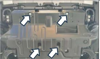
3. Remove OEM under panel by undoing four M8 Bolts. Retain for refitment.
