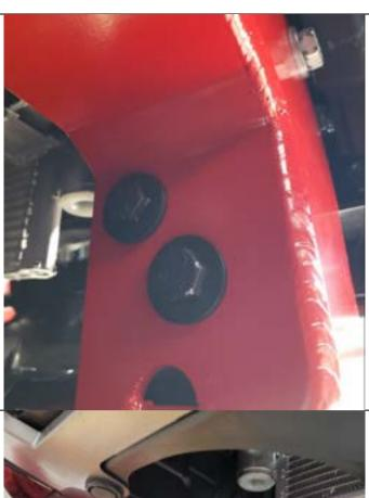
20. Loosely assemble two M8x110 bolts and hardened washers from the rear and fasten with flange nuts.
