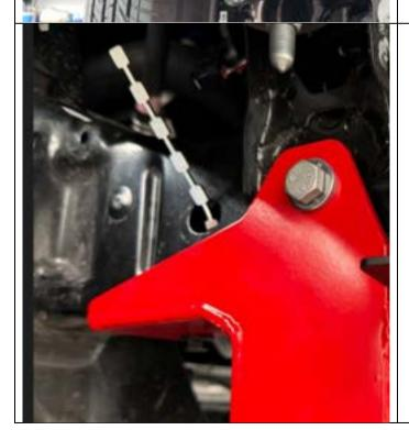
23. Install nut plate through chassis hole and fasten M12x1.75x50 flange bolt as shown. Break off nut plate tail using vice grips or similar and re-install plastic chassis cover removed in Step 8.
