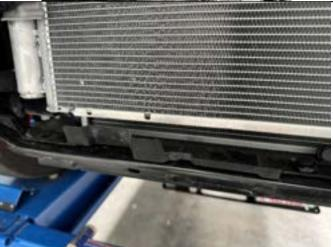
Remove plastic trim panel underneath cooling stack by removing five scrivets and disengaging moulded clip. Retain for refitment.
