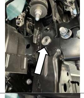
16. Identify and assembly M8 crush tube into chassis hole shown.
