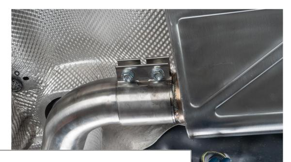
Join the front and middle sections of the catback together using the included exhaust clamp and 15mm socket.
