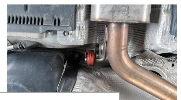
Remove the exhaust from the OE hanger by using either an exhaust hanger removal tool, or a pry bar.
