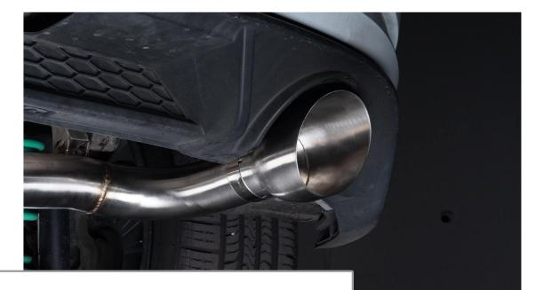
Slide the two Exhaust tips into place on the rear section of the catback. Adjust to your preferred depth with the bumper then tighten in place using a 12mm socket.
