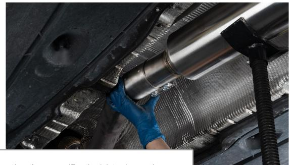
Raise the front portion of your new iE catback into place and secure it to the downpipe using the appropriate exhaust clamp. For now, simply hand tighten the exhaust clamp. You will tighten after final adjustments have been made.
