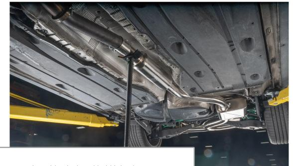
Support the center section with a jack and hold it in place as you move from the front of vehicle to the rear and adjust, then tighten each exhaust clamp to 42 ft/lbs. Do a couple passes to ensure that fitment is correct.
