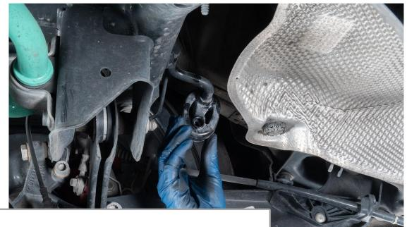
Install the supplied rubber exhaust hanger on the OE hanger location on the drivers side just in front of the rear sway bar. Some silicone lubricant may help with this.
