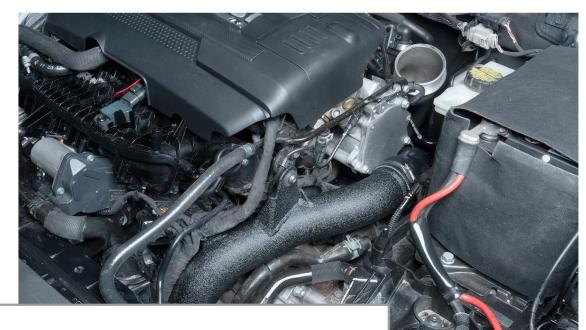
Lower the chargepipe into the engine bay and connect the hose to the turbo. You will then reinstall all mounting hardware, intake and belly pan in reverse order.
