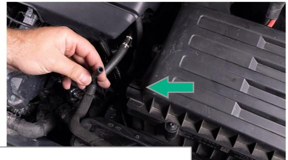
Unplug vacuum hose from stock air box by pulling it straight out.
