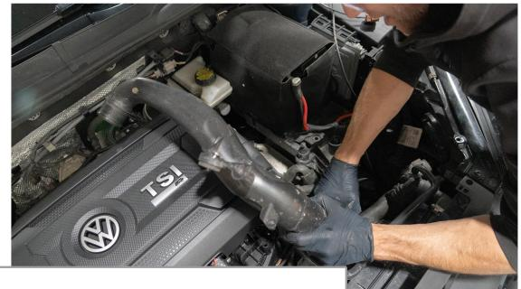
The OE Chargepipe should now be free and able to be pulled out. You will need to twist and finagle the pipe a bit to pull it out the top. Pay attention to not get it caught on any wiring or hoses.
