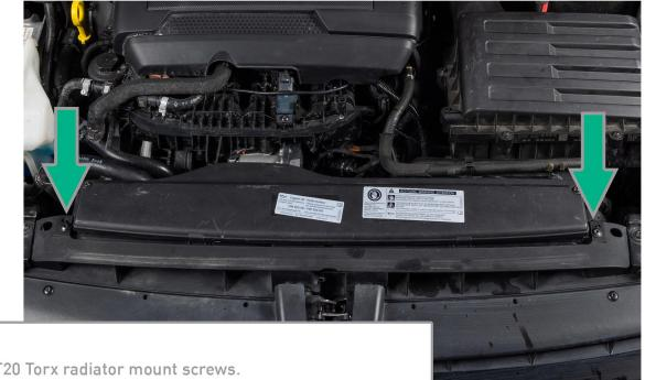
Remove two T20 Torx radiator mount screws.
