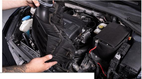
Pull straight up on stock air box to release from two rubber grommets and remove from vehicle.
