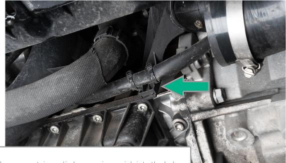
Remove wiring harness retainer clip by pressing a pick into the hole on the back side and pulling straight down.
