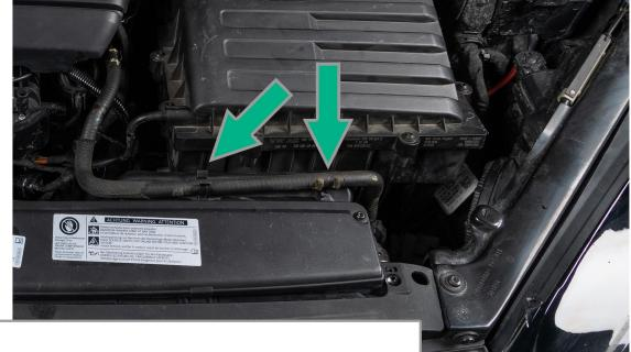
Pull up on upper coolant line to release from two hose clips.
