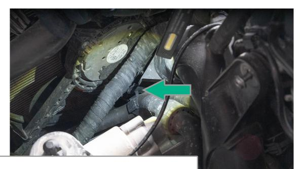
Using a trim removal tool, pop out coolant hose retainer.
