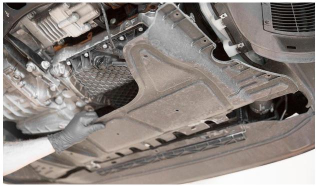
Remove the T25 torx screw from the underside of the bumper that secures it to the radiator
