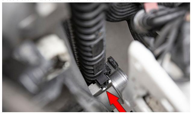
Line up the upper radiator clips with the slots on the IE intercooler, push to clip into place.
