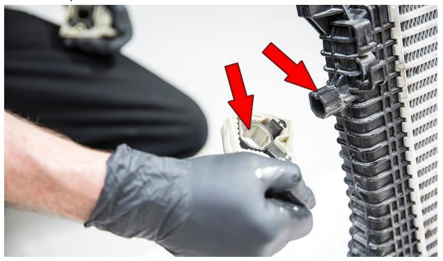
Reinstall the mount brackets in the same orientation onto your new IE intercooler.
