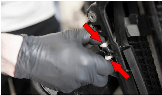
Press down on the radiator securing tabs from the top of the intercooler with a flat head screwdriver and pull the radiator away from the IC.
