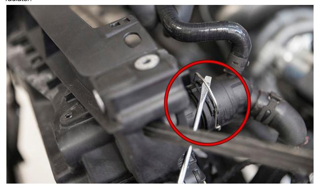
Remove the three connectors from the radiator support. There are two yellow connectors and one black connector located at the top of the radiator support. Be sure there are no electrical connectors still attached to the radiator support.
