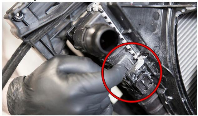
With the radiator fan disconnected, pull up to remove it from the vehicle.
