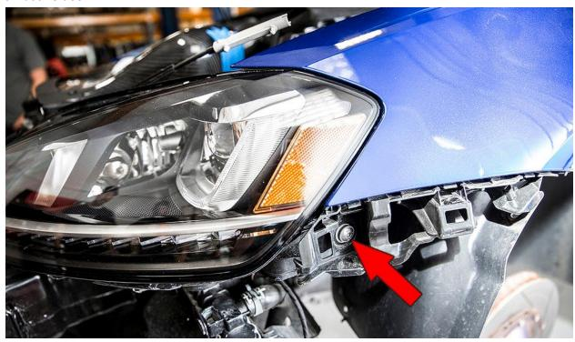
Remove the two T30 torx screws from the engine bay side of the headlight.
