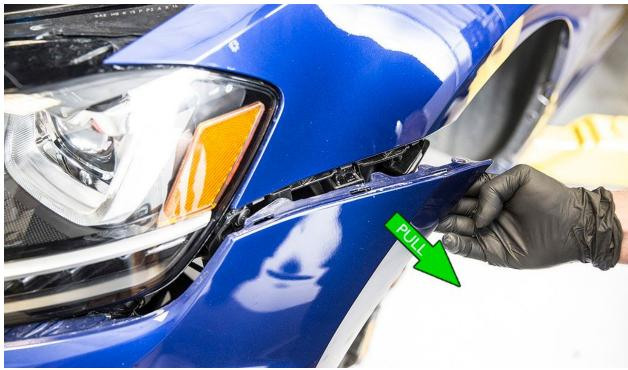
Pull the front bumper forward and disconnect any/all electrical connectors for fog lights, air temperature, parking sensors, etc...
