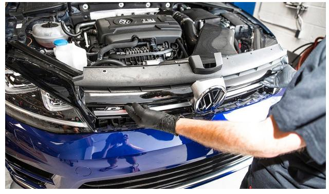
Remove three T30 torx screws in the center to release the bumper from the radiator support bracket.
