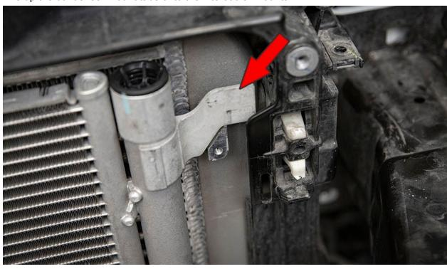
Install the included condenser brackets and button head allen bolts with a 3mm allen.
