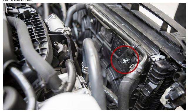
Disconnect the cooling fan connector.
