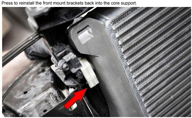
Slide the radiator into the bottom radiator mounts on the IE intercooler.
