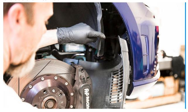
Be sure to remove the torx located under the fender liner towards the top of the bumper. Repeat on both sides.
