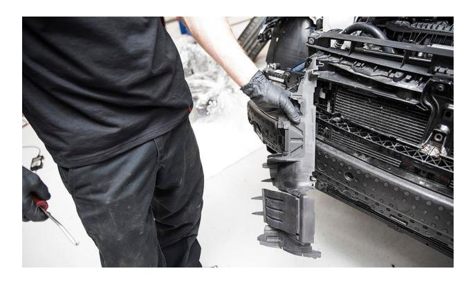
To fully remove the bumper support bracket, remove the two T30 torx screws remaining on the outside of the support. Release the two push tabs on the inside of the support. Be careful when removing to not break plastic components on the bumper support bracket.
