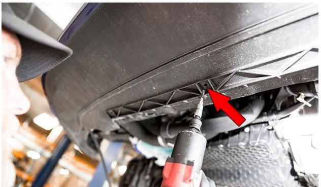
Remove the T25 torx screws in the wheel well that secure the front bumper. You can now remove the lower wheel liners.
