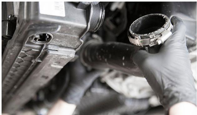
Remove the spring clip from the lower radiator hose.
