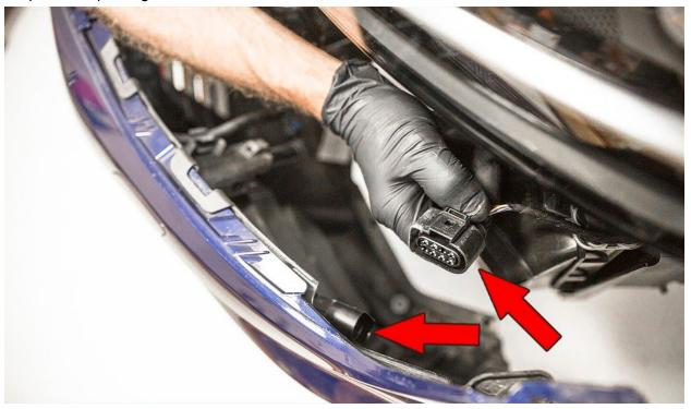
With all electrical connectors disconnected, carefully remove the bumper as set aside.
