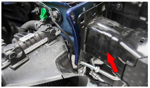
Remove the two T30 screws securing the coolant pipe located in front of the intake manifold to the radiator fan.
