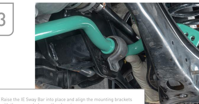
with the proper holes on the chassis.
