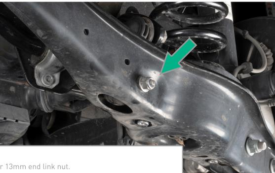
Remove the lower 13mm end link nut.
