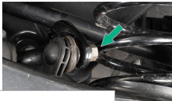
Remove 16mm End Link Nuts that connect the end links to the OE Sway Bar.
