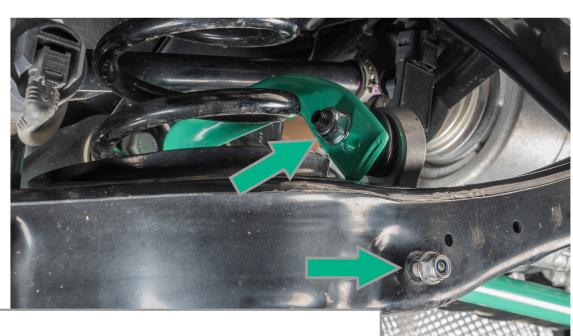
Align and reinstall lower end link bolt and nut, along with the upper end link nut. Torque the upper nut to 55 ft lbs.
