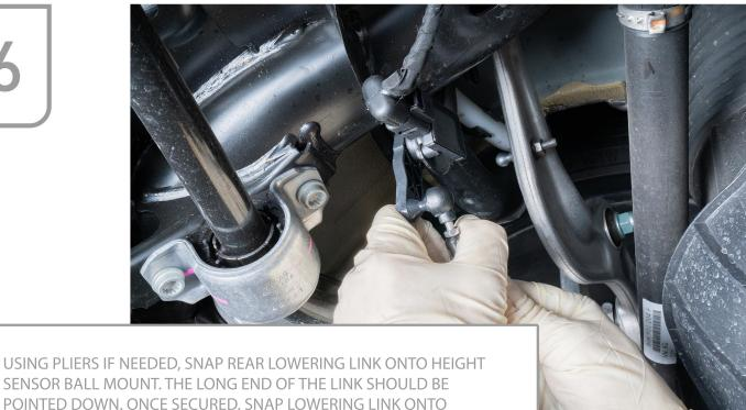
SENSOR BALL MOUNT. THE LONG END OF THE LINK SHOULD BE POINTED DOWN. ONCE SECURED, SNAP LOWERING LINK ONTO CONTROL ARM BALL MOUNT.
