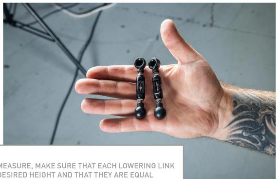
USING A TAPE MEASURE, MAKE SURE THAT EACH LOWERING LINK IS SET TO THE DESIRED HEIGHT AND THAT THEY ARE EQUAL LENGTHS. REAR LINKS WILL BE LONGER THAN FRONT LINKS.
