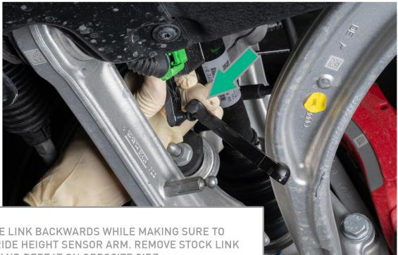
GENTLY PRY THE LINK BACKWARDS WHILE MAKING SURE TO SUPPORT THE RIDE HEIGHT SENSOR ARM. REMOVE STOCK LINK FROM VEHICLE AND REPEAT ON OPPOSITE SIDE.
