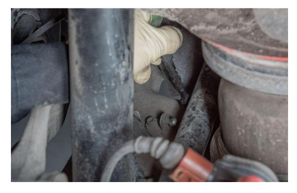
While supporting the ride height sensor arm, pop off the upper mount of the OEM link. Do so by applying pressure upwards.
