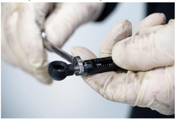
Apply a dab of the supplied grease to the inside of both mounting points of IE links.
