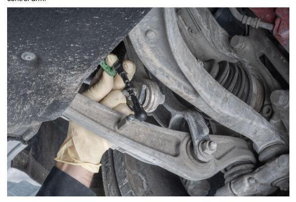
While supporting the ride height sensor arm, pop off the upper mount of the OEM link. Do so by applying pressure upwards while supporting the ride height sensor arm.
