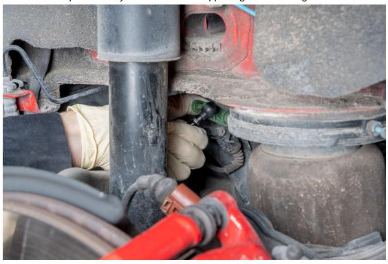
Press on the lower mount of the IE link to the control arm mounting point.
