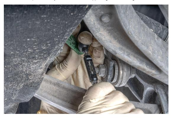
Press on the lower mount of the IE link to the mounting point on the control arm.
