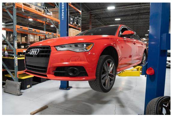
Use a 17mm socket to remove the rear wheels to gain access to the OEM rear links.
