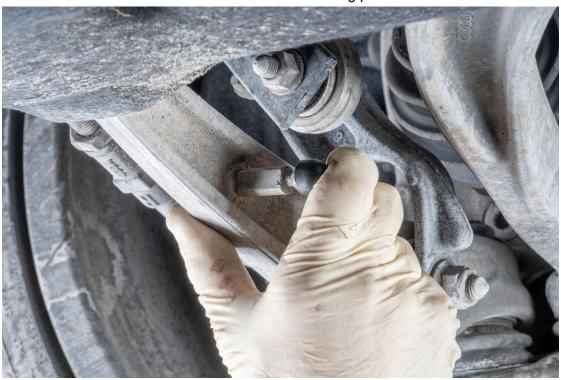
Locate the rear OEM Links and begin by popping off the lower mount that is attached to the control arm.
