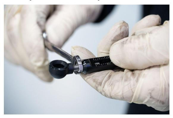
Apply supplied grease to the inside of both mounting points of IE links.
