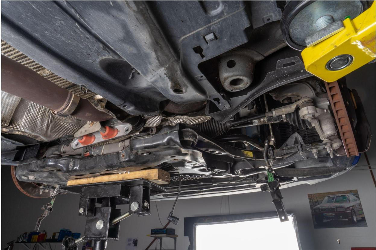
Remove oem sway bar by gently pulling down on subframe while lifting the sway over the top mount of the subframe and out the front
