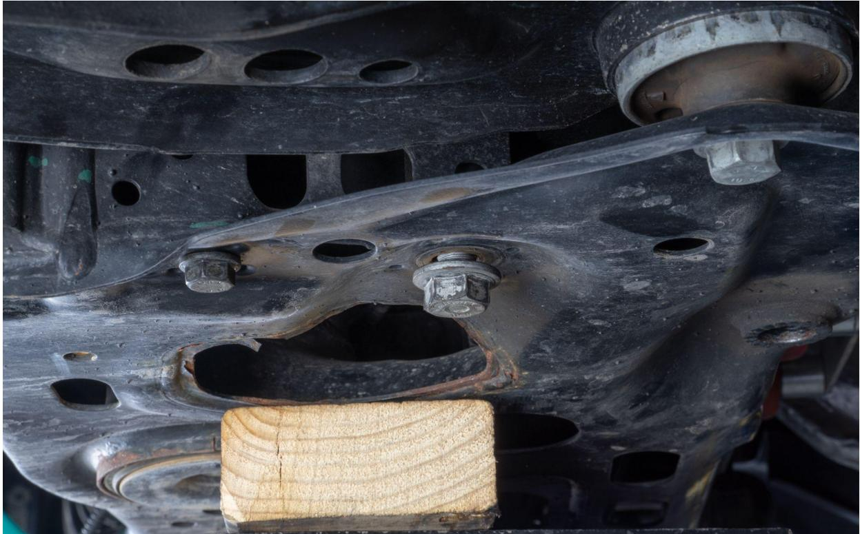
When attaching the end links to the sway bar, take note that the front mounting location will yield a softer roll, while the rear will yield a stiffer roll.
