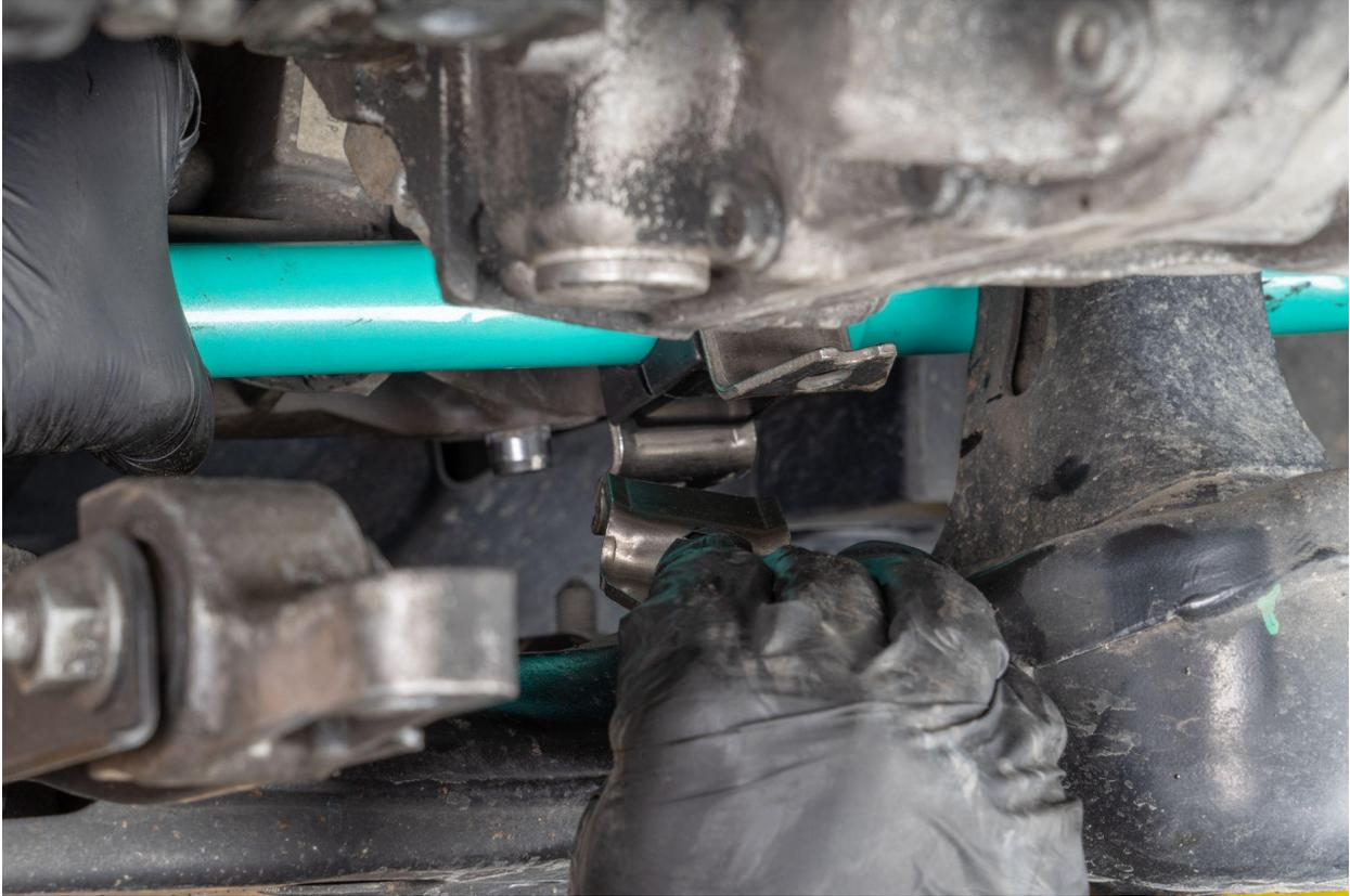
Align top and bottom mount plates with the two sway bar mount bolts that pass through the subframe, then hand tighten nuts onto bolts.
