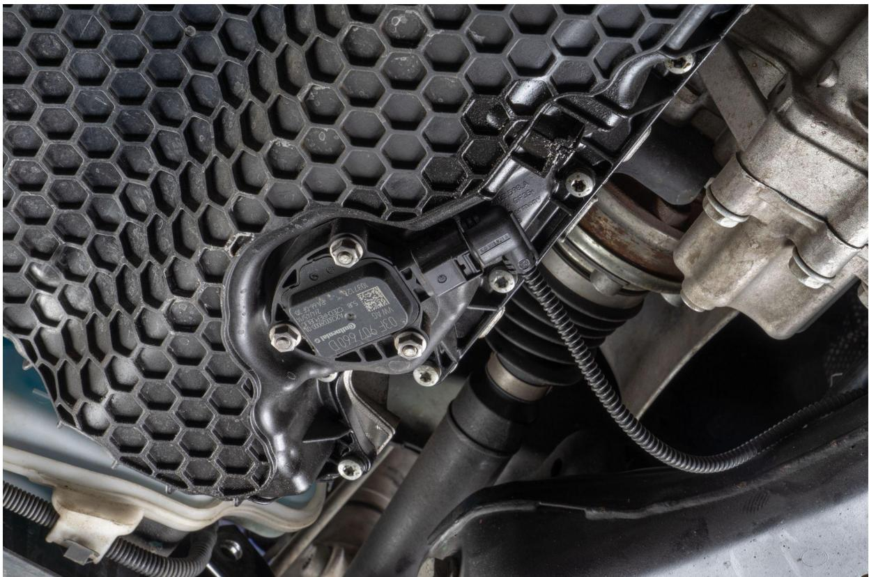
Follow the wires from the Oil Level Sensor til you find the wire retainer clip, then press it out of the subframe.
