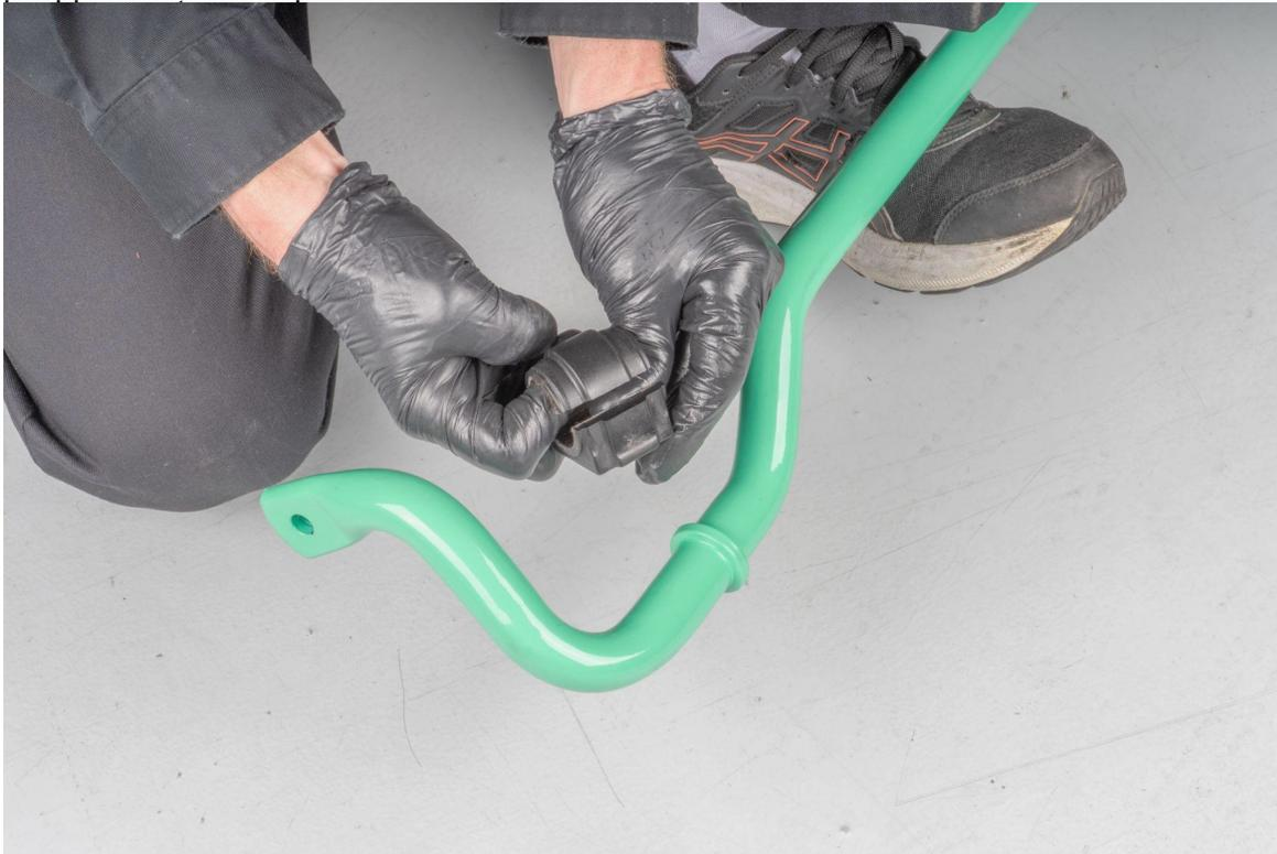
Pictured below is the proper position of the bushings once installed.
