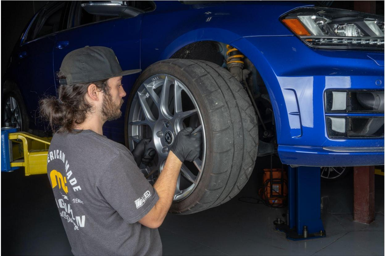
Remove lower end link nuts using M6 triple square and an 18mm wrench
