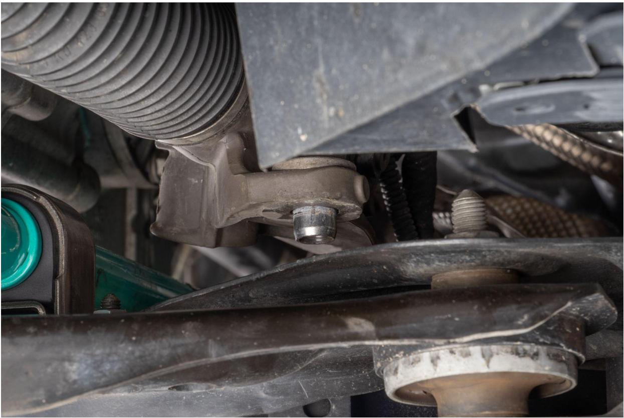
Finger thread all hardware for the subframe before lifting into its final location, then torque all subframe and steering rack hardware to factory spec. (Specs listed at bottom of install guide) Take care to not cross thread body mount bolts.
