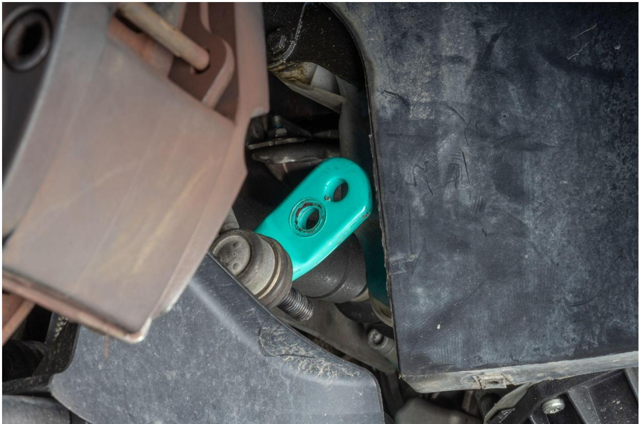
When tightening the sway bar brackets, make note that the sway bar is clear of the steering rack on the drivers side. A pry bar through the subframe to provide pressure while tightening can help with this. Finish the install by reversing install instructions for all hardware, sensor mounts, and wheels. Enjoy the look and feel of your new IE Performance Sway Bar!
