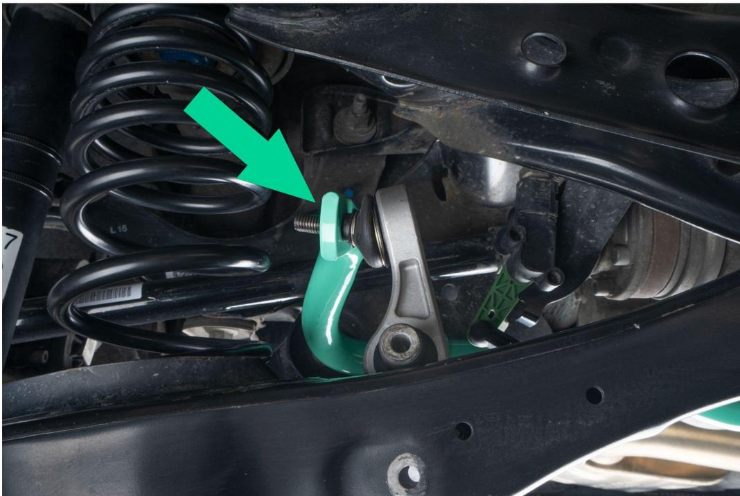
Loosely Install 17MM nut onto end link
