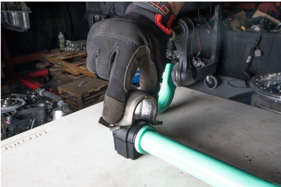
Reinstall old links on new IE sway bar using a 16MM wrench and M6 triple square.
