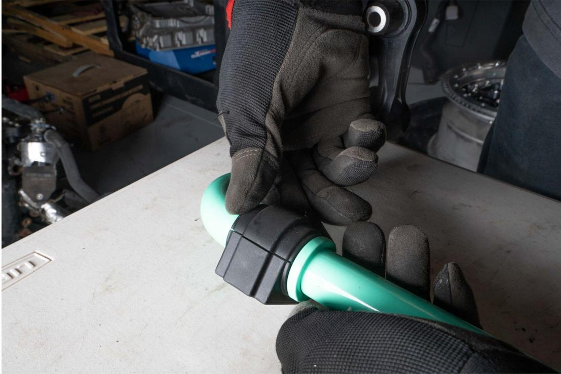
Install sway bar mounting bracket onto new IE sway bar.
