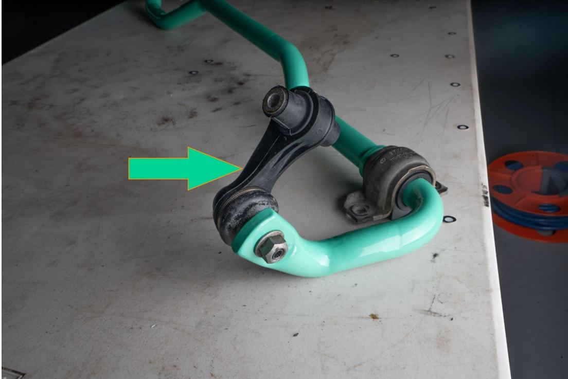
Lift sway bar into place over exhaust and around differential onto the sub frame.
