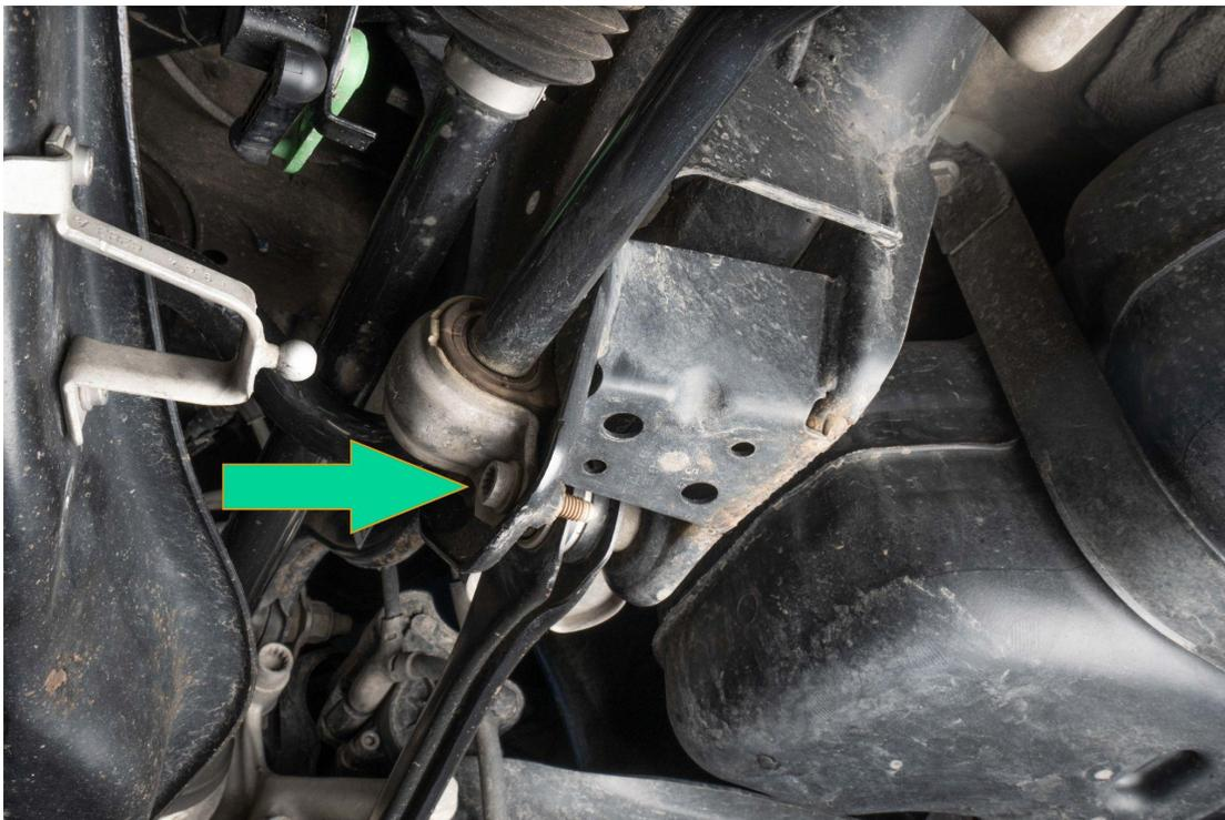
Use a jack to support the lower control arm and remove the lower control arm 18MM bolt and lower shock 18MM bolt.
