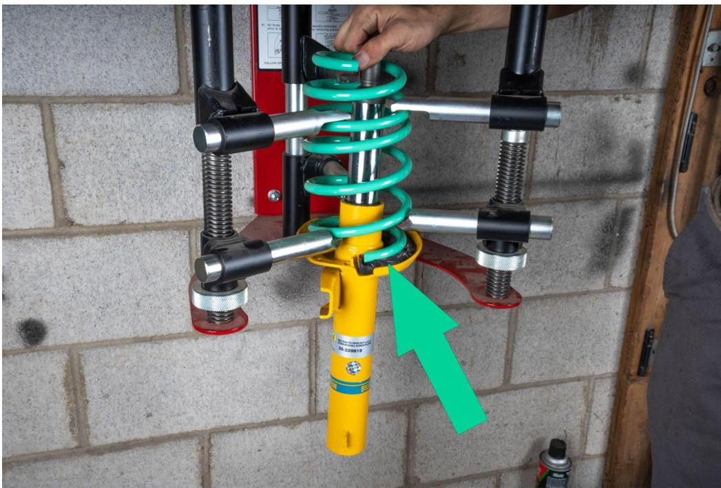
Assemble upper spring perch and strut mount on top of the shock and secure nut to strut mount
