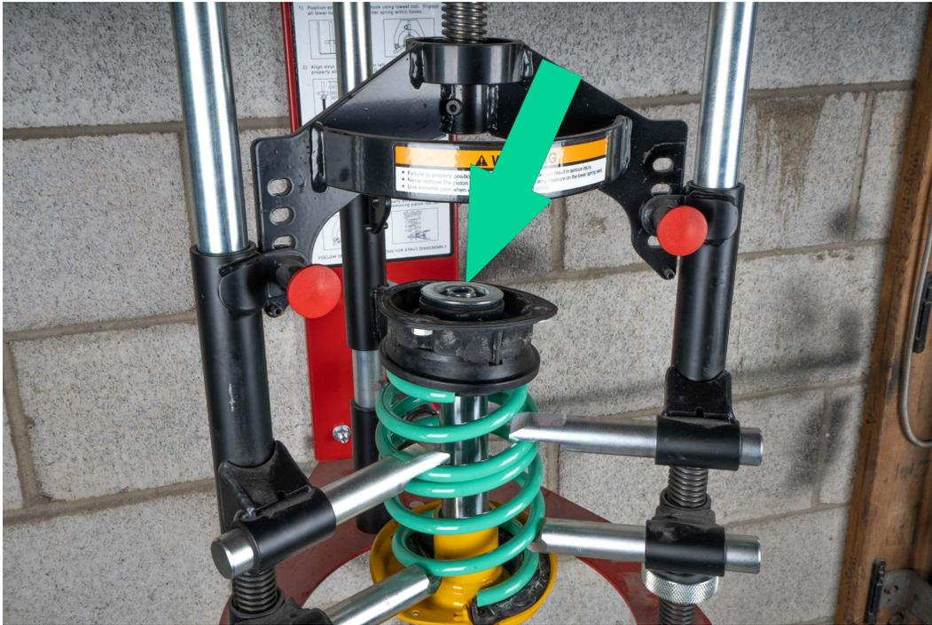
Once nut is secure, remove entire assembly from spring compressor
