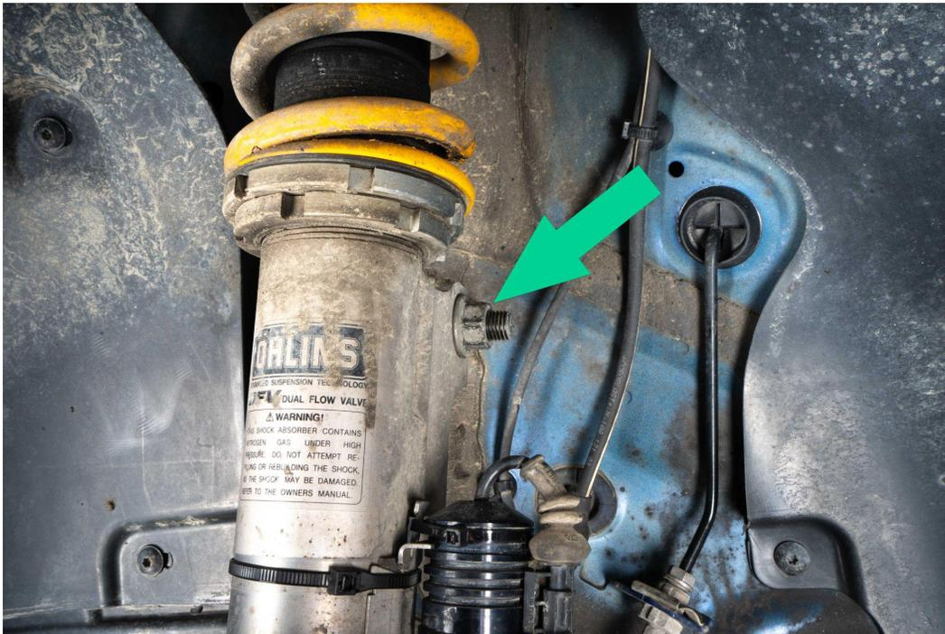
Use an M14 triple square to remove strut bolt, and an 18mm socket to remove nut
