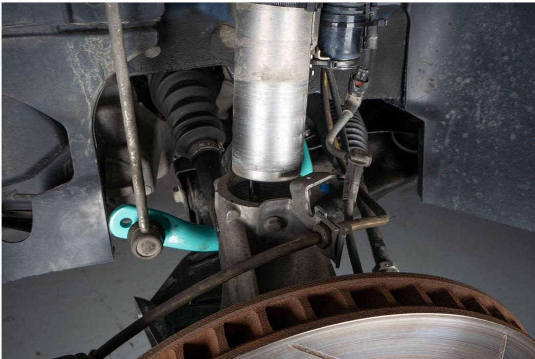
Lift rain tray to access upper strut mount bolts on strut tower
