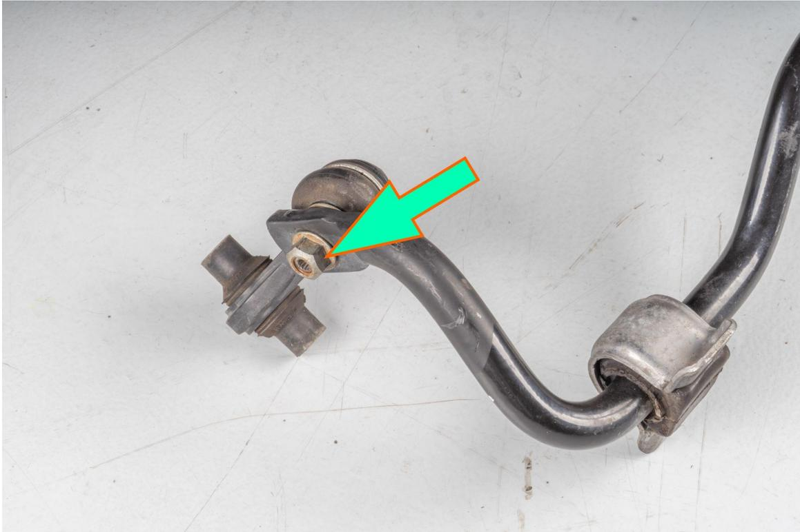
Open and liberally lubricate inside and outside of the bushing, then install rubber sway bar bushings on the sway bar
