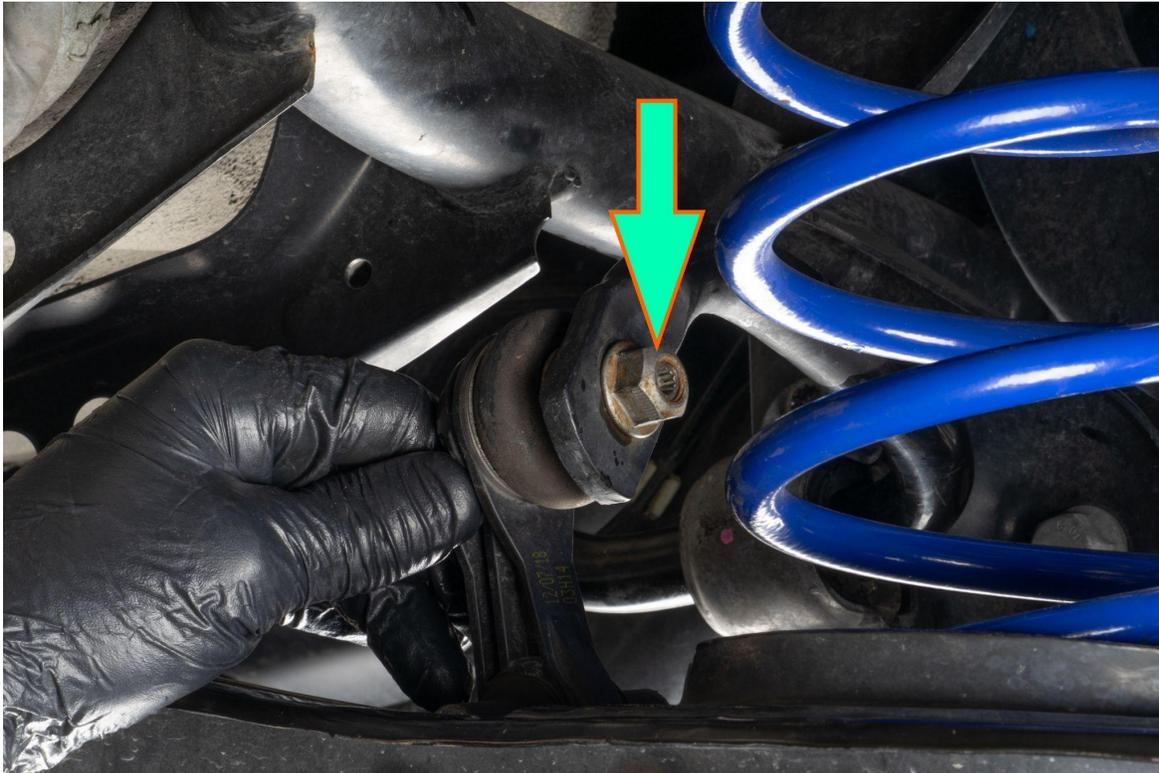
Using triple square #10 remove 4 sway bar mount bolts
