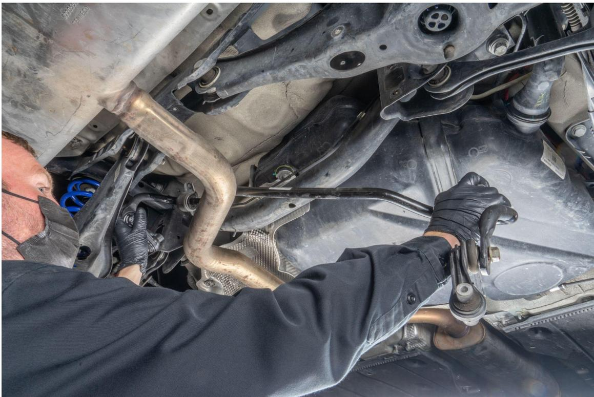
Use it a triple square #6 hold sway bar link stud in place and use 16mm wrench to loosen nut
