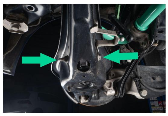
Disconnect the ride height sensor by pulling straight away from mounting point.
