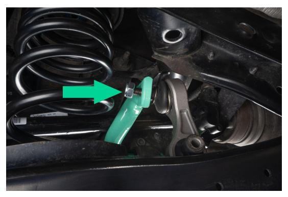
Lower end link to align with hole on lower control arm and Install 13mm bolt connecting end link and lower control arm
