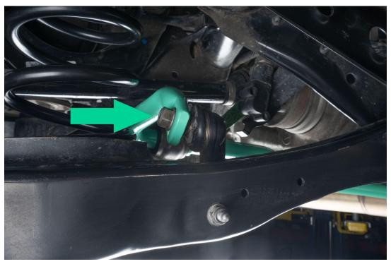
Remove 13MM nut and bolt securing end link to lower control arm using a 13MM socket and Wrench
