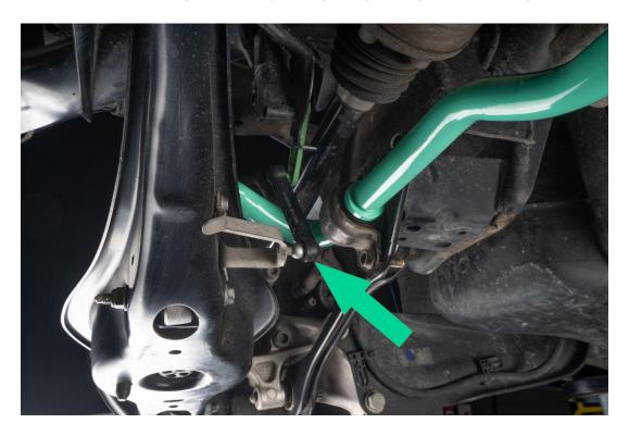
Slightly loosen the sway bar mount bolts using an M10 triple square
