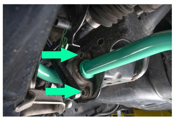
Install 13mm nut onto bolt connecting the end link and lower control arm
