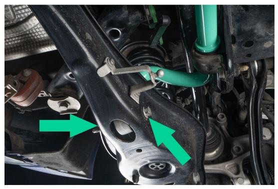
Secure all hardware to end links using 17mm wrench and a 5mm Allen
