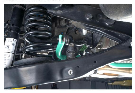
Set new end links in place with the bolt facing outwards
