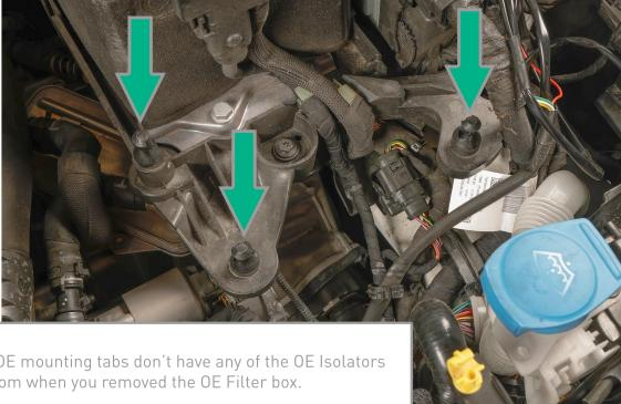
Ensure that the OE mounting tabs don't have any of the OE Isolators stuck on them from when you removed the OE Filter box.
