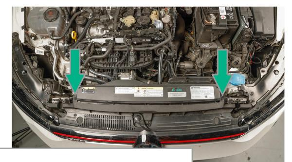
Remove the two T25 Screws that secure the OE Inlet
