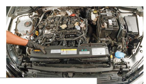
Remove OE Intake Inlet from the engine bay.
