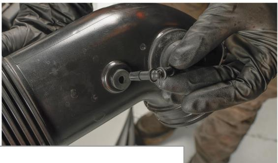
Insert the 90 degree vacuum hose barb into the bottom of the intake tube, then install the vaccum line into place.
